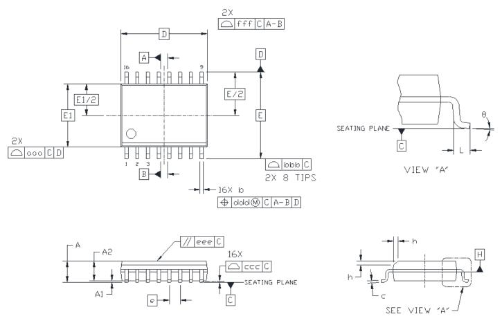
Figure 6.3. 16-Pin Wide Body SOIC Package
