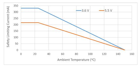
Figure 4.2. Thermal Derating Curve for Safety Limiting Current (DIP8)
