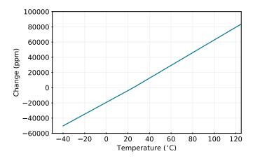
Figure 4.11. Normalized Differential Input Resistance vs. Temperature
