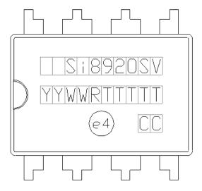
Figure 6.5. Si8920 DIP8 Top Marking
