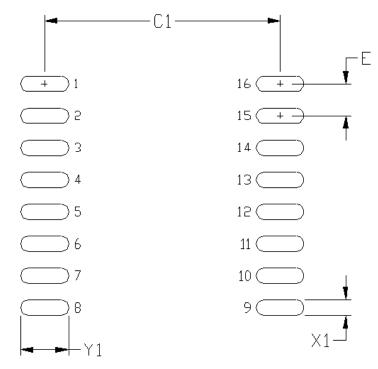
Figure 6.4. 16-Pin Wide Body SOIC Land Pattern
