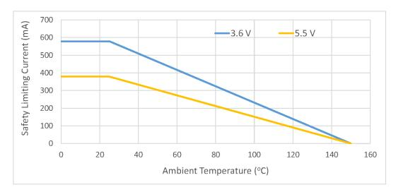
Figure 4.3. Thermal Derating Curve for Safety Limiting Current (WB SOIC-16)
