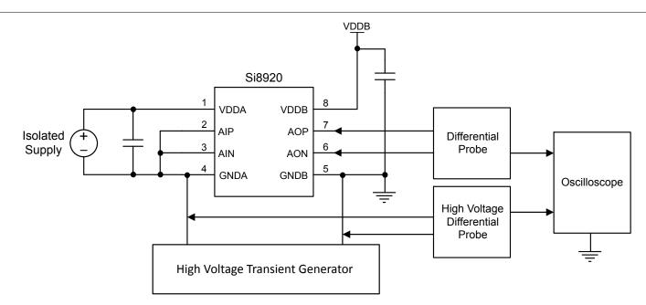
Figure 4.1. Common-Mode Transient Immunity Characterization Circuit
