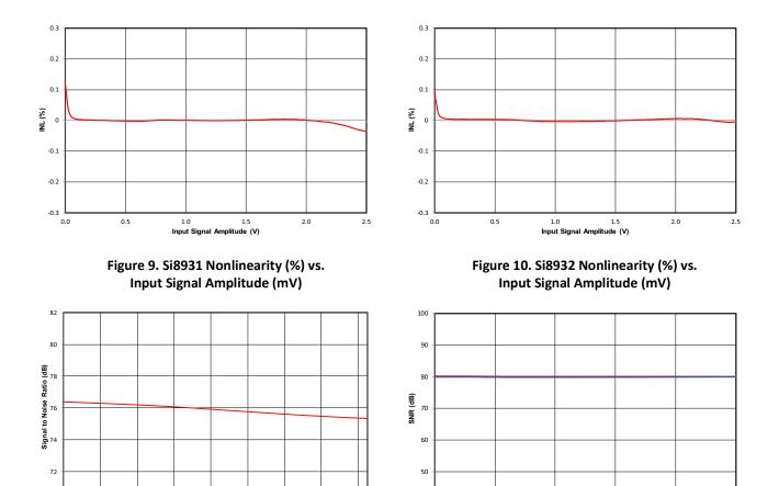
Figure 11. Signal-to-Noise Ratio (dB) vs. Temperature (°C)
