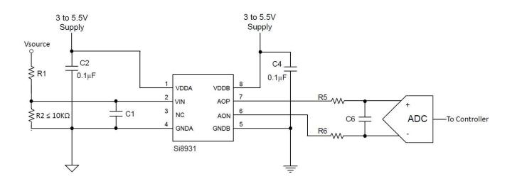
Figure 5. Voltage Sense Application
