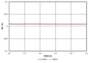
Figure 8. Nonlinearity (%) vs. VDDA Supply (V)
