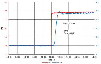
Figure 32. Si8932 Low-to-High Step Response
