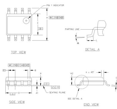
Figure 40. 8-Pin Narrow Body SOIC Package
