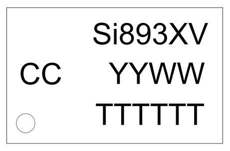
Figure 42. Si8931/32 Typical Package Marking, 8-Pin Narrow Body SOIC
