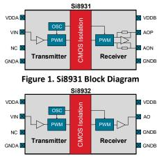
Figure 2. Si8932 Block Diagram
