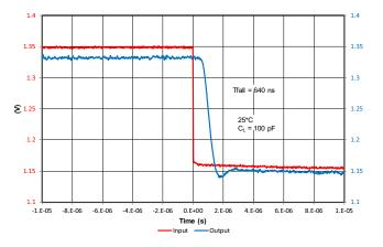
Figure 31. Si8932 High-to-Low Step Response
