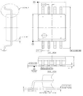
Figure 35. 8-Pin Wide Body Stretched SOIC Package
