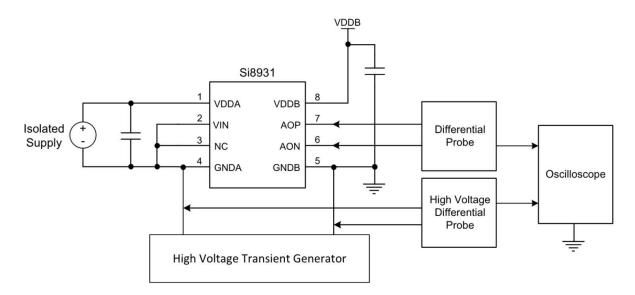
Figure 6. Common-Mode Transient Immunity Characterization Circuit
