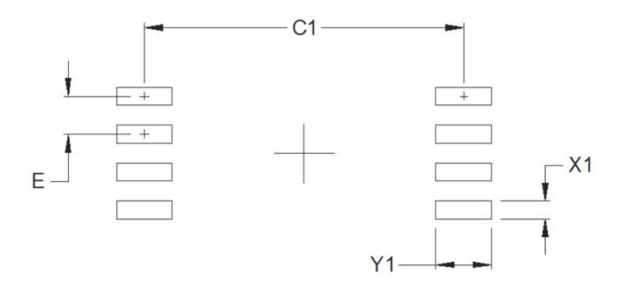
Figure 36. 8-Pin Wide Body Stretched SOIC Land Pattern
