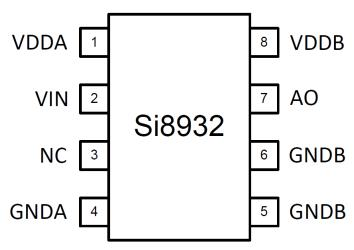
Figure 4. Si8932 Pinout (Top View)
