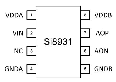
Figure 3. Si8931 Pinout (Top View)
