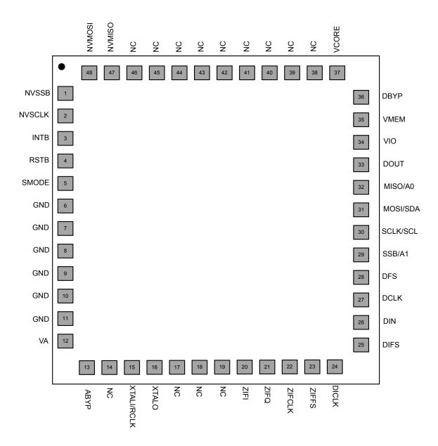
Figure 1.1. 48-pin QFN
