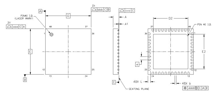
Figure 2.1. 48-Pin QFN
