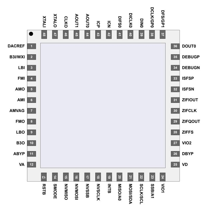
Figure 1.1. Si47901-02 Pinout Diagram
