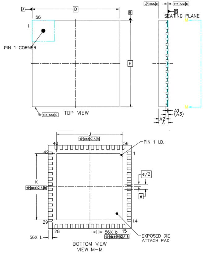
Figure 2.2. 56-Pin QFN
