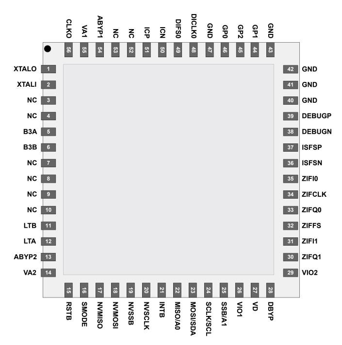
Figure 1.1. Si47942 Pinout Diagram
