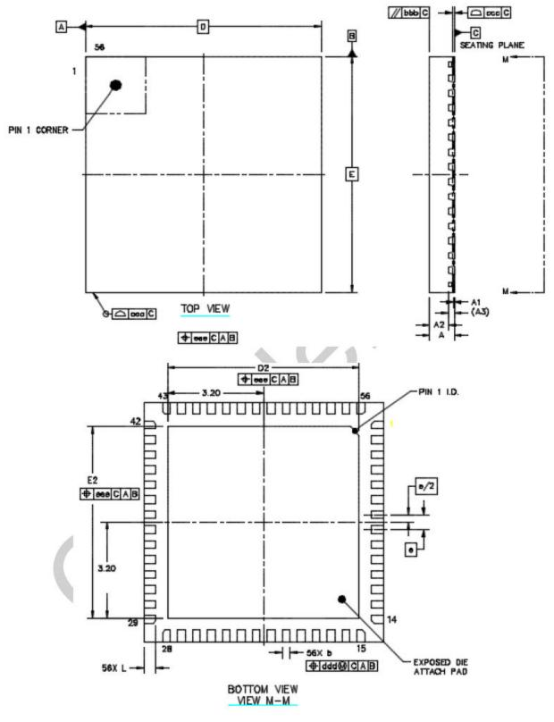
Figure 2.1. 56-Pin QFN
