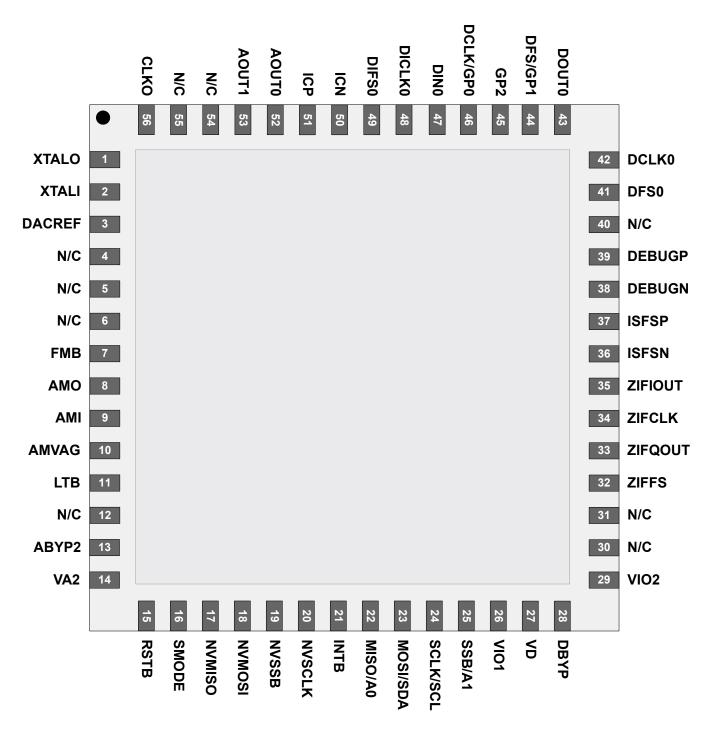
Figure 1.1. Si47957 Pinout Diagram
