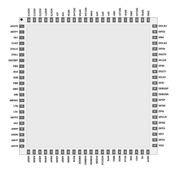
Figure 1.1. Si47971-72 Pinout Diagram
