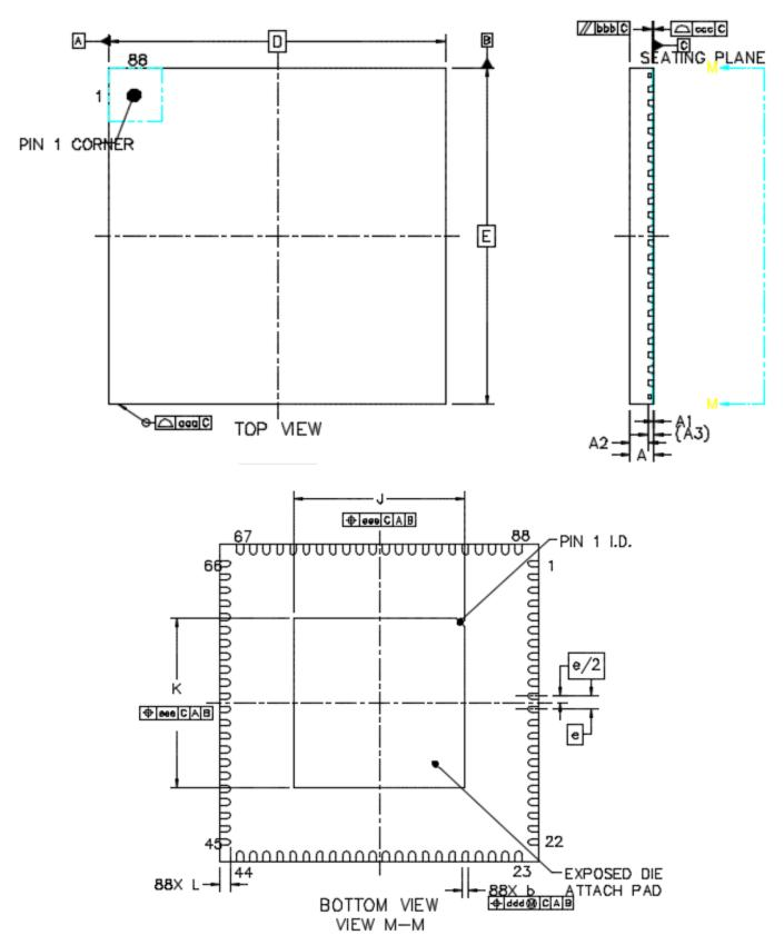
Figure 2.2. 88-Pin QFN
