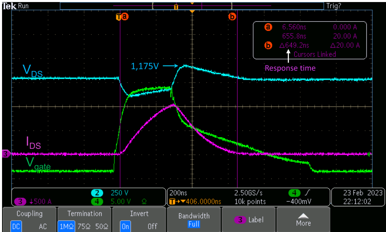
Figure 19. Si8281 DESAT Waveform with V_{Rail} = 800\text{ V} , R_{SS} = 33\ \Omega , and C3M0016120K SiC
