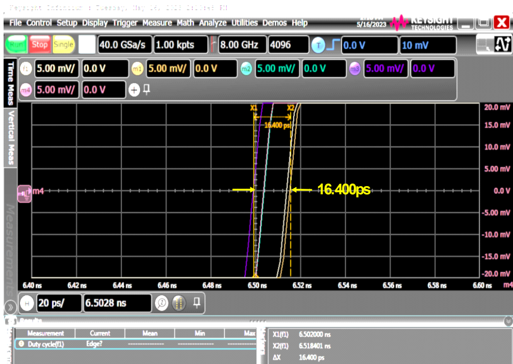
Figure 17. Sample Output-to-Output Skew for LVPECL Output
