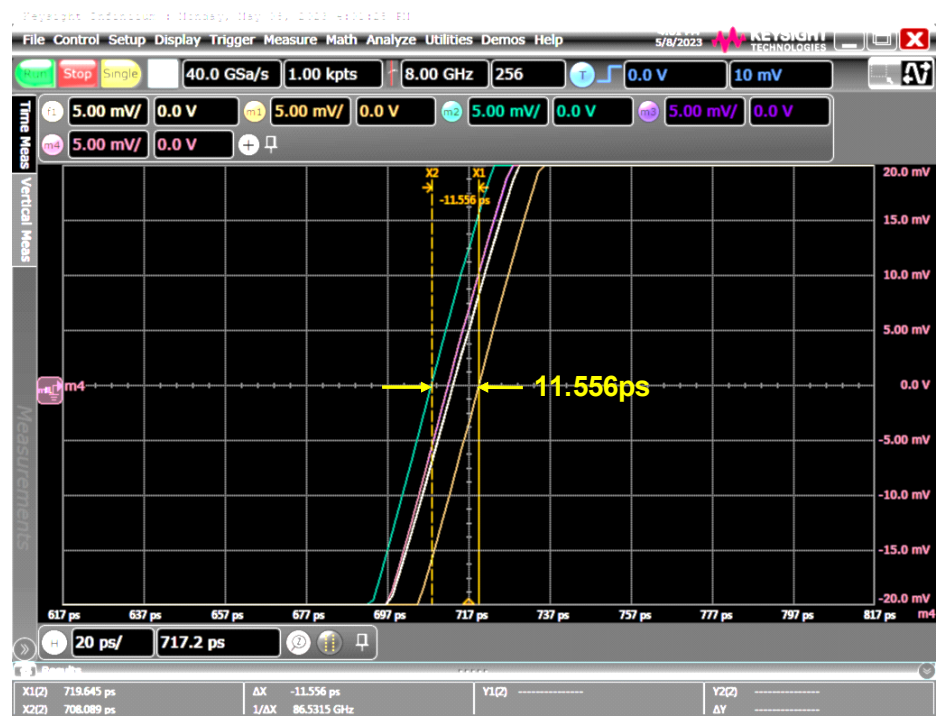
Figure 18. Sample Output-to-Output Skew for LVDS Output
