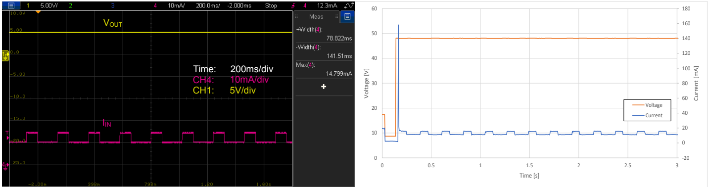
Figure 5.11. Si3406-Buck Non-Isolated EVB, 5 V, Class 2 PD Automatic Maintain Power Signature (MPS) Generation
