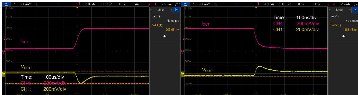
Figure 6.5. Si3406-Buck Non-Isolated EVB, 12 V, Class 2 PD Output Load Step Transient Test
