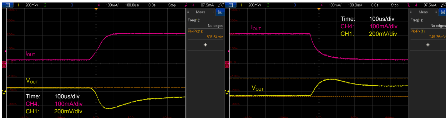
Figure 7.5. Si3406-Buck Non-Isolated EVB, 24 V, Class 2 PD Output Load Step Transient Test
