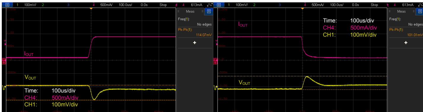
Figure 5.5. Si3406-Buck Non-Isolated EVB, 5 V, Class 2 PD Output Load Step Transient Test
