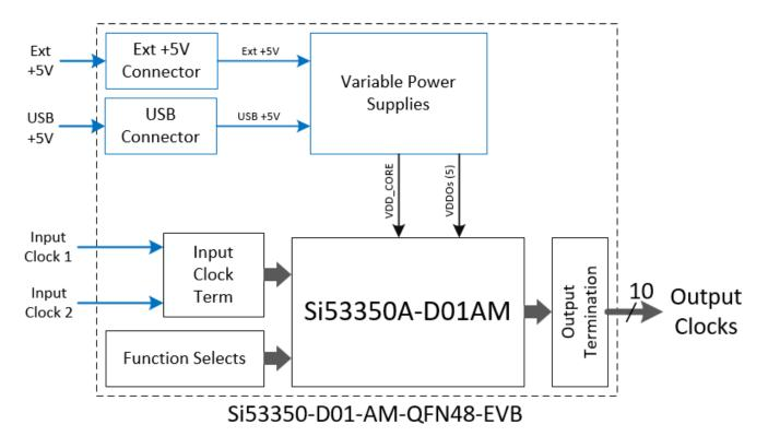
Figure 1.1. Si53350-D01-AM-QFN48-EVB Functional Block Diagram
