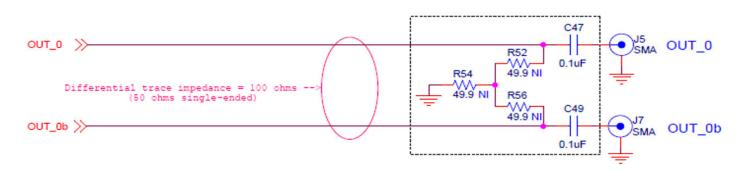
Figure 5.1. Si53350-D01-AM-QFN48-EVB Output Clock Termination Circuit
