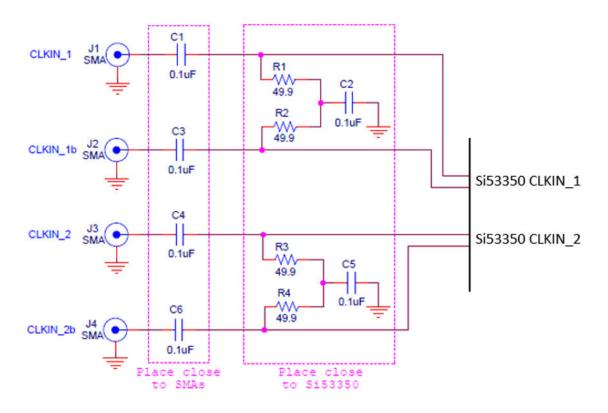
Figure 4.1. Si53350-D01-AM-QFN48-EVB Input Clock Termination Circuit
