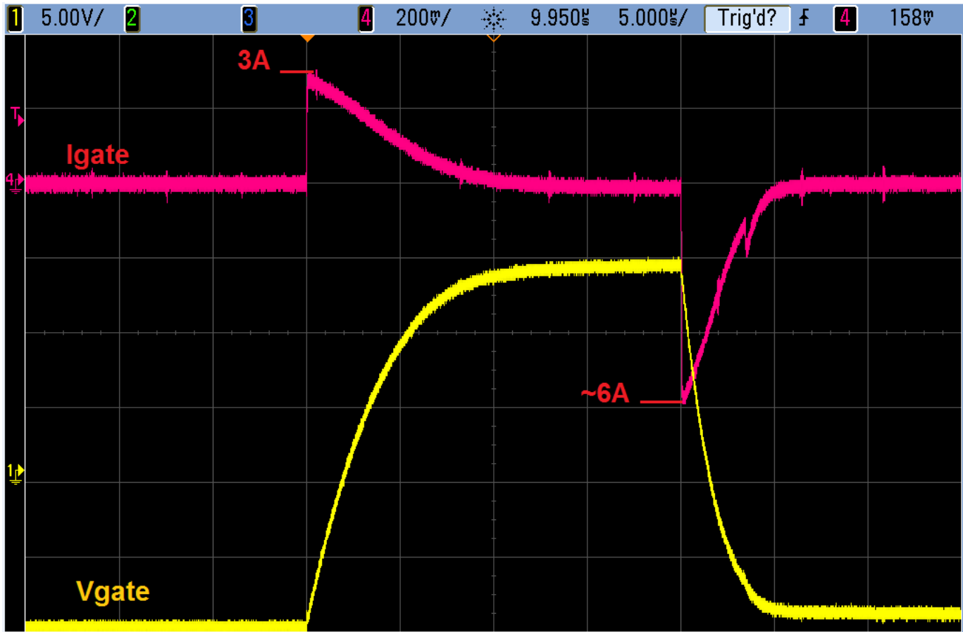
Figure 2.3. Standard Gate Drive Response
