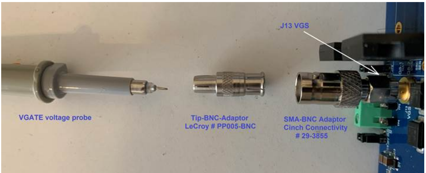
Figure 2.6. Connection for VGS Scope Probe at J13
