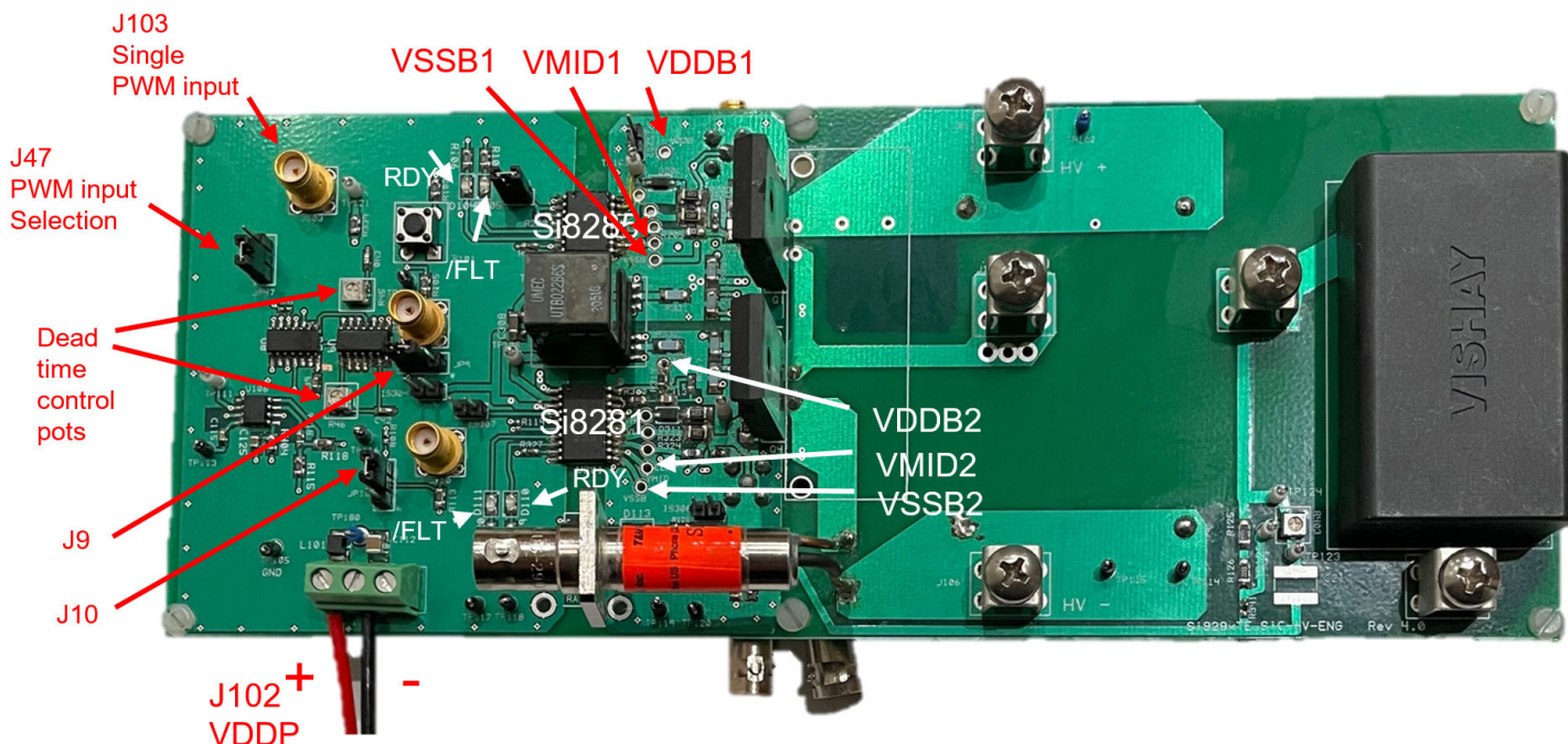
Figure 2.1. Si828x-HB-EVB Input Power and Input Signals
