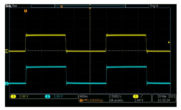
Figure 2.1. Si86SS41 Transmitting a 500 kHz (3 Vpeak) Signal through the Si86SS41
