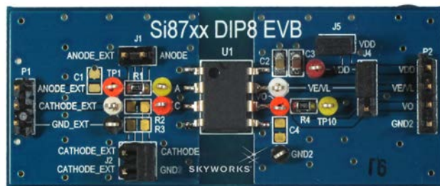
Figure 1. Si87xx DIP8 Evaluation Board Overview
