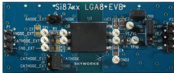
Figure 4. Si87xx LGA8 Evaluation Board Overview
