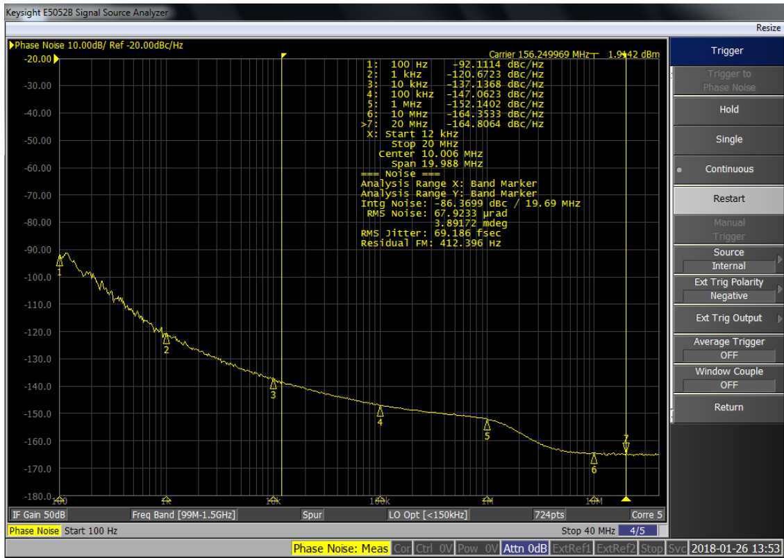
Figure 4.2. Phase Noise Plot Si5395P RMS Jitter 12 kHz–20 MHz Integration Band
