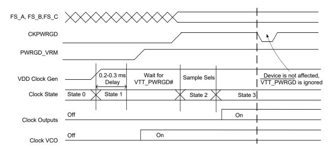
Figure 3. CKPWRGD Timing Diagram
