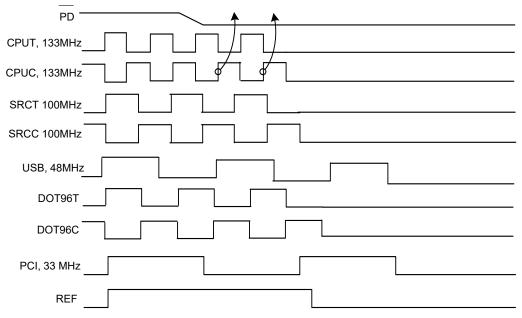
Figure 1. Powerdown Assertion Timing Waveform
