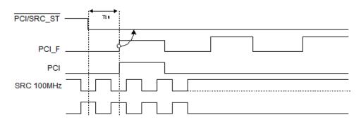
Figure 6. PCI/SRC\_STP# Assertion Waveform
