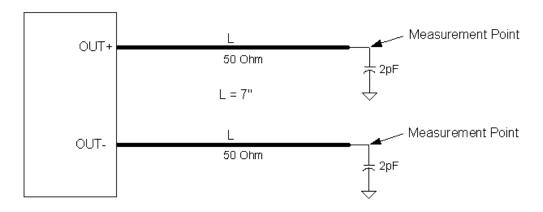
Figure 10. 0.7 V Differential Load Configuration
