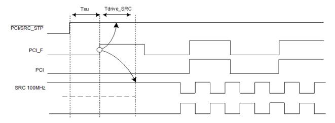
Figure 7. PCI/SRC\_STP# Deassertion Waveform
