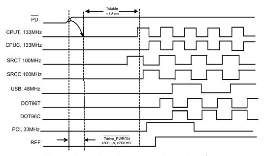
Figure 2. Powerdown Deassertion Timing Waveform
