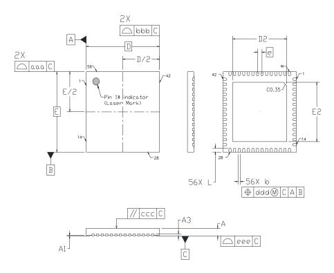
Figure 13. 56-Lead QFN Package
