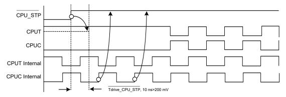
Figure 5. CPU STP# Deassertion Waveform
