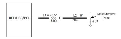
Figure 8. Single-ended Clocks Single Load Configuration
