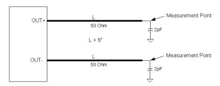
Figure 1. 0.7V Differential Load Configuration
