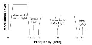
Figure 11. MPX Signal Spectrum
