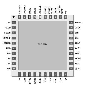
Figure 23. Si4777 Pin Descriptions for IBOC Blend Mode
