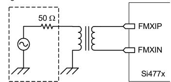
Figure 5. FM Test Circuit for Mixer Input IP3 and Sensitivity Measurement
