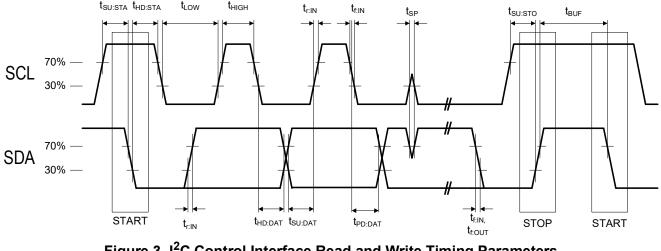
Figure 3. I<sup>2</sup>C Control Interface Read and Write Timing Parameters
