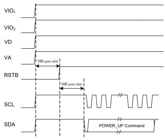
Figure 27. Startup Timing
