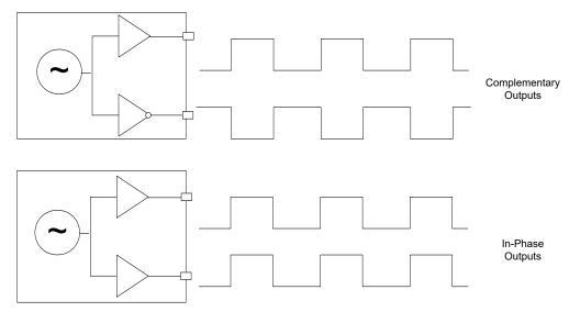
Figure 1. Integrated 1:2 CMOS Buffer Supports Complementary or In-Phase Output
