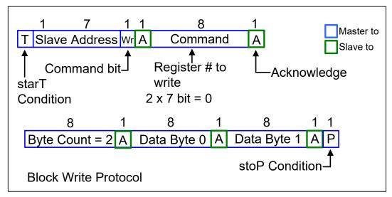
Figure 11. Block Write Protocol
