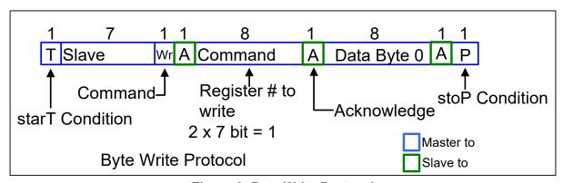
Figure 9. Byte Write Protocol
