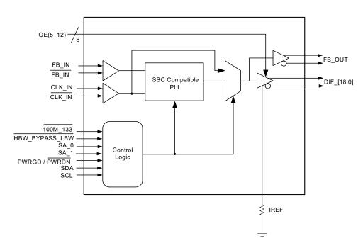
Figure 1. Si53019-A01A Functional Block Diagram
