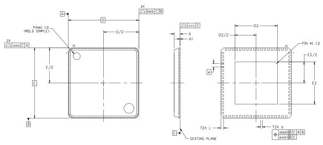
Figure 13. 72-Pin Quad Flat No Lead (QFN) Package
