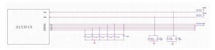
Figure 12. Schematic Example of the Si53019-A01A Power Filtering
