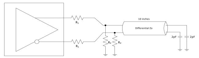
Figure 7. 0.7 V Configuration Test Load Board Termination
