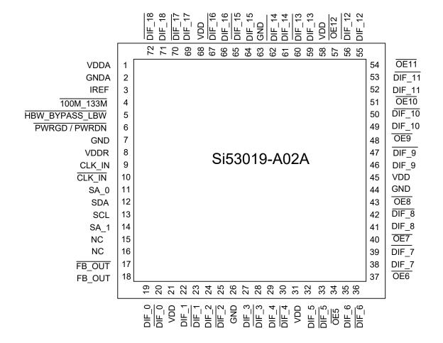
Note: FB\_OUT pins must be identically terminated to the other DIF outputs.
