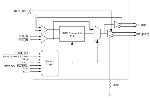
Note: FB\_OUT pins must be identically terminated to the other DIF outputs.
