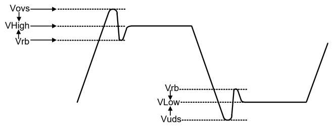
Figure 5. Single-ended Measurement Points for  $V_{ovs}$ ,  $V_{uds}$ ,  $V_{rb}$
