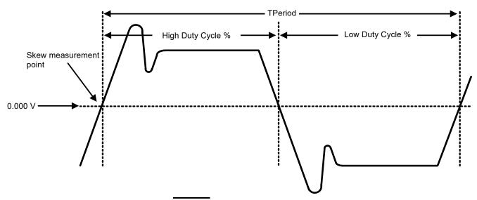
Figure 6. Differential (CLOCK-CLOCK) Measurement Points (Tperiod, Duty Cycle, Jitter)
