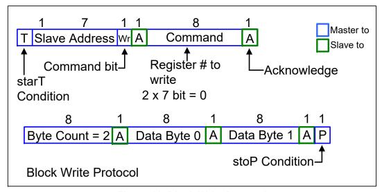
Figure 11. Block Write Protocol
