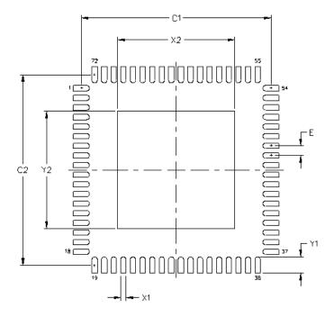
Figure 14. 72-Pin Quad Flat No Lead (QFN) Package
