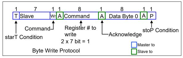
Figure 9. Byte Write Protocol
