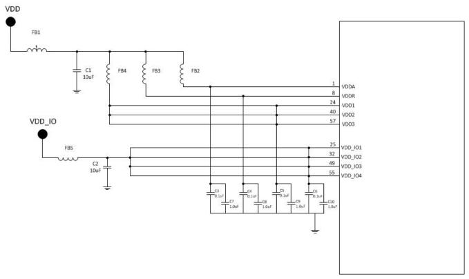
Figure 12. Schematic Example of Si53112 Power Filtering
