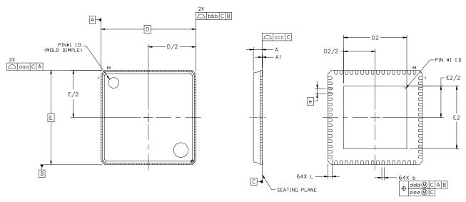
Figure 13. 64-Pin Quad Flat No Lead (QFN) Package
