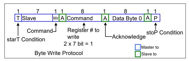
Figure 9. Byte Write Protocol
