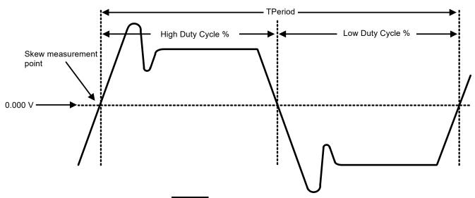
Figure 6. Differential (CLOCK–CLOCK) Measurement Points (T<sub>period</sub>, Duty Cycle, Jitter)
