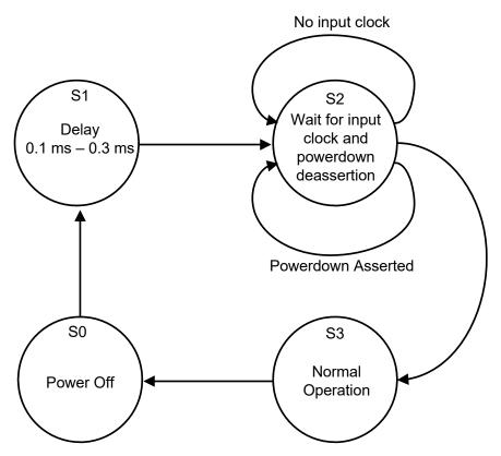
Figure 3. Buffer Power-Up State Diagram
