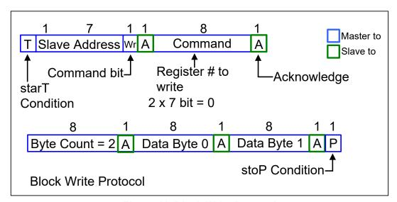
Figure 11. Block Write Protocol
