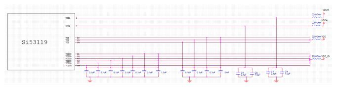
Figure 11. Schematic Example of the Si53119 Power Filtering
