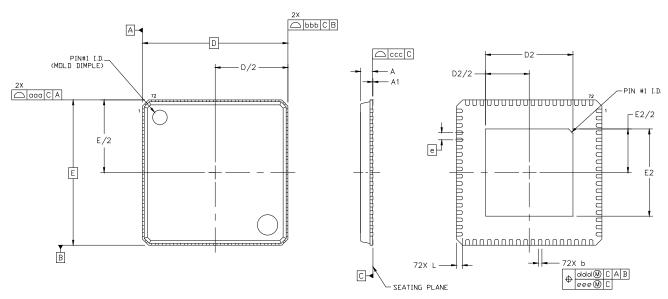
Figure 12. 72-Pin Quad Flat No Lead (QFN) Package
