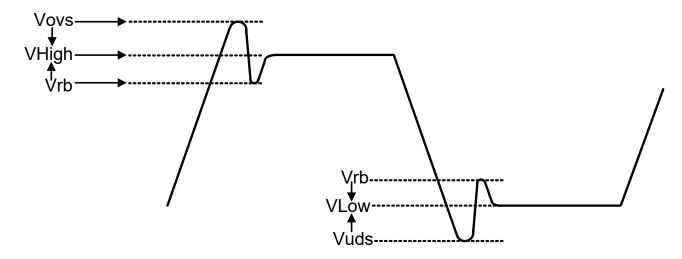
Figure 4. Single-Ended Measurement Points for  $V_{ovs}$ ,  $V_{uds}$ ,  $V_{rb}$
