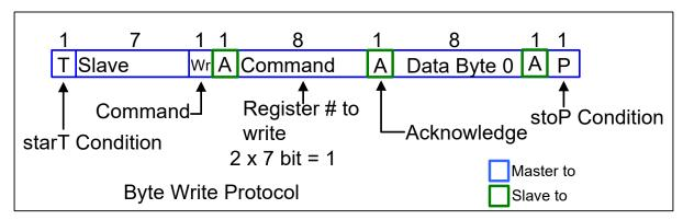
Figure 8. Byte Write Protocol
