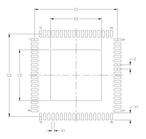
Figure 13. 72-pin QFN Land Pattern
