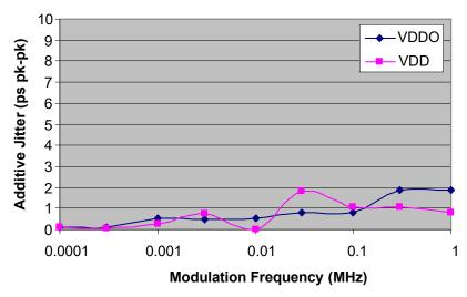
Figure 6. Peak-to-Peak Additive Phase Jitter from 100 mV Sine Wave on Supply
