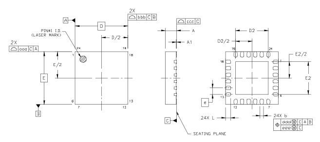
Figure 7. 24-Lead Quad Flat No-Lead (QFN)
