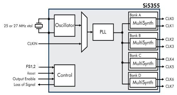
Figure 1. Si5355 Functional Block Diagram
