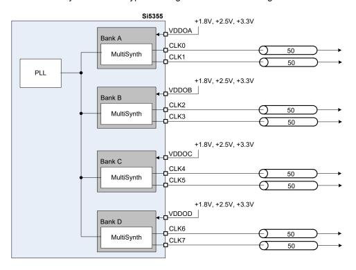
Figure 5. CMOS Output Driver Configuration
