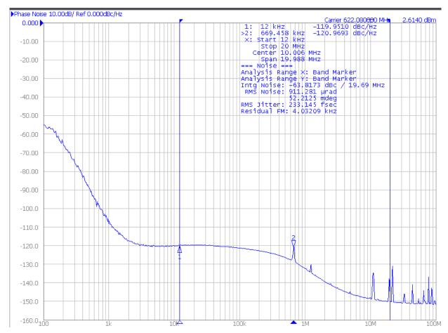
Figure 3. Typical Phase Noise Plot
