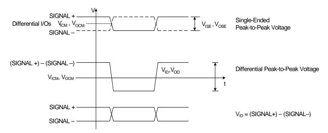
Figure 1. Differential Voltage Characteristics
