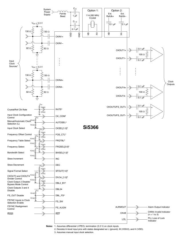
Figure 4. Si5366 Typical Application Circuit
