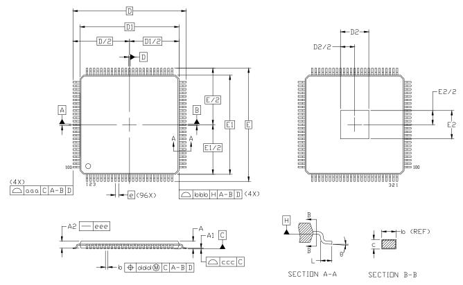
Figure 5. 100-Pin Thin Quad Flat Package (TQFP)
