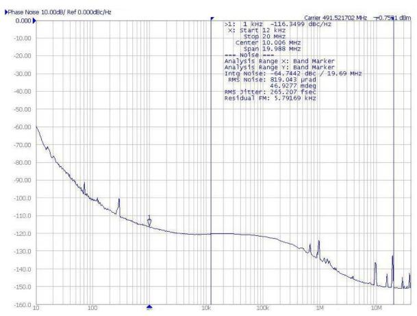
Figure 5. Wireless Base Station Phase Noise\*
