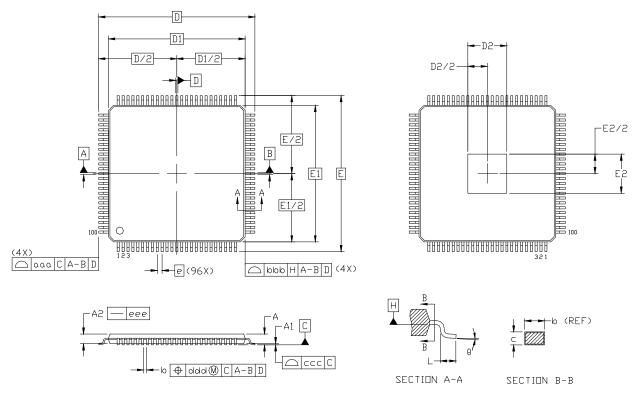
Figure 9. 100-Pin Thin Quad Flat Package (TQFP)
