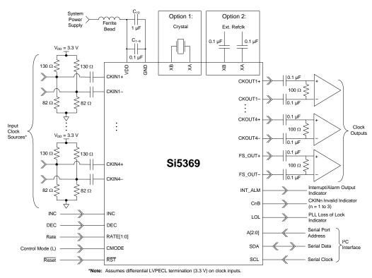
Figure 7. Si5369 Typical Application Circuit (I<sup>2</sup>C Control Mode)
