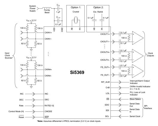
Figure 8. Si5369 Typical Application Circuit (SPI Control Mode)
