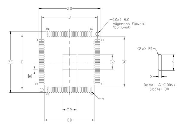
Figure 10. PCB Land Pattern Diagram
