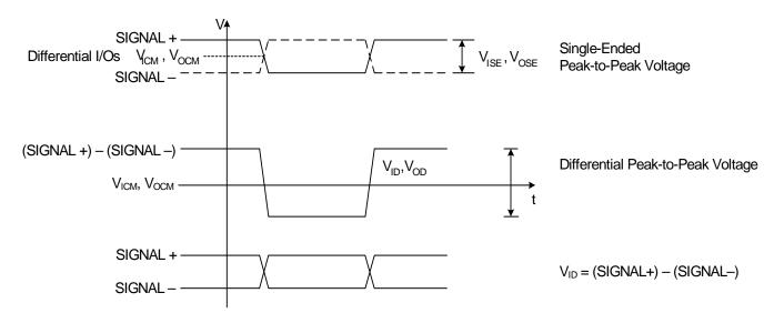
Figure 1. Differential Voltage Characteristics
