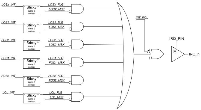
Figure 5. Si5374 Alarm Structure
