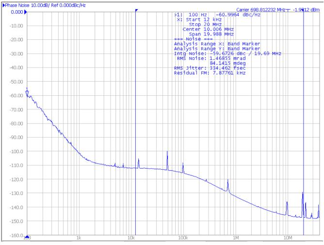
Figure 3. Typical Phase Noise Plot
