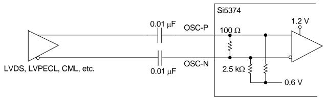
Figure 6. Differential OSC Reference Input Example for Si5374
