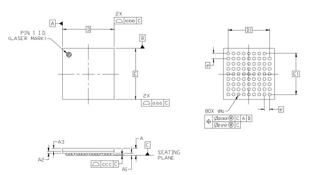
Figure 10. 80-Pin Plastic Ball Grid Array (PBGA)
