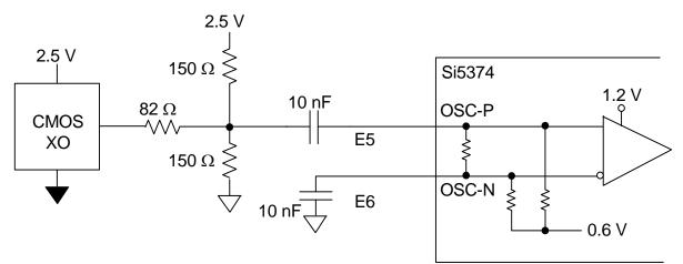
Figure 8. Single-Ended, 2.5 V, CMOS XO Connection
