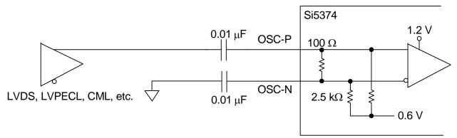
Figure 7. Single-Ended OSC Reference Input Example for Si5374
