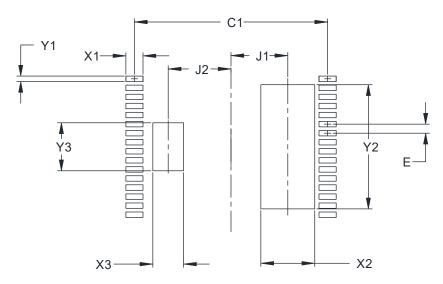
Figure 37. Recommended Land Pattern Details for the Si834x in a 32-pin 9x9 DFN Package
