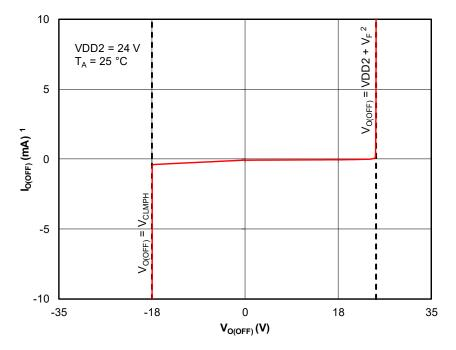
Figure 34. OFF State Output Current (I<sub>O(OFF)</sub>) vs. Output Voltage (V<sub>O(OFF)</sub>) for Sourcing Devices<sup>1,2</sup>
