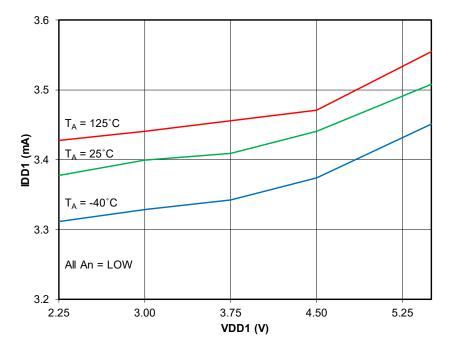
Figure 30. Logic Interface Supply Quiescent Current (IDD1<sub>Q</sub>) vs. Logic Interface Supply Voltage (VDD1)
