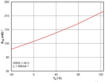
Figure 29. On Resistance ( $R_{ON}$ ) vs. Ambient Temperature ( $T_A$ )<sup>1,2</sup>
