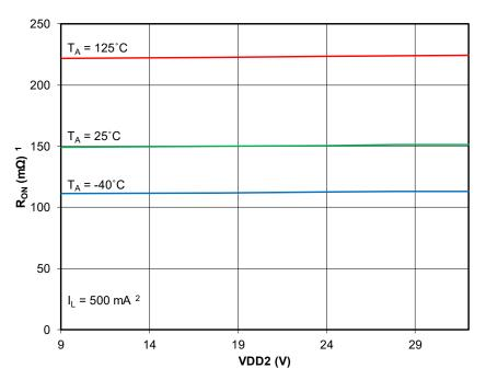
Figure 28. On Resistance (R<sub>ON</sub>) vs. Switch Supply Voltage (VDD2)<sup>1,2</sup>
