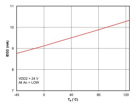
Figure 33. Switch Supply Quiescent Current (IDD2<sub>Q</sub>) vs. Ambient Temperature (T<sub>A</sub>)
