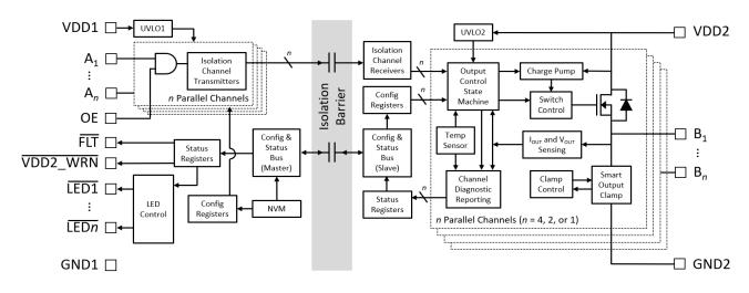
Figure 3. Parallel Interface Device System Diagram
