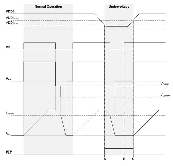
Figure 15. VDD1 Undervoltage Shutdown Behavior
