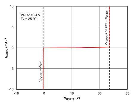
Figure 35. OFF State Output Current ( $I_{O(OFF)}$ ) vs. Output Voltage ( $V_{O(OFF)}$ ) for Sinking Devices<sup>1,2</sup>
