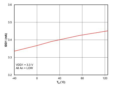
Figure 31. Logic Interface Supply Current Quiescent (IDD1<sub>Q</sub>) vs. Ambient Temperature (T<sub>A</sub>)
