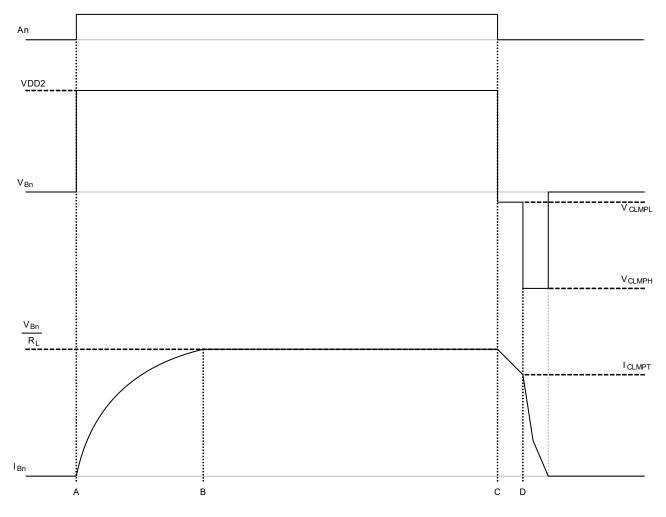
**Figure 8. Demagnetization Protection Behavior**
