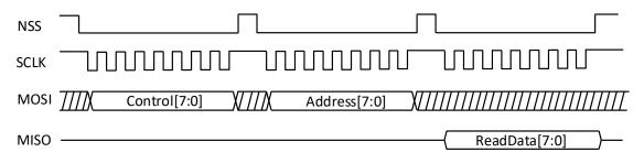
Figure 17. SPI Read Operation
