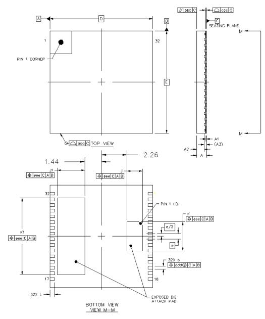
Figure 36. Si834x in 32-Pin 9x9 DFN (DFN-32)
