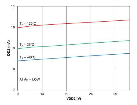
Figure 32. Switch Supply Quiescent Current (IDD2 $_{\rm Q}$ ) vs. Switch Supply Voltage (VDD2)
