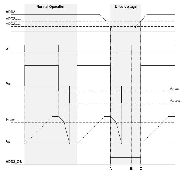
Figure 14. VDD2 Undervoltage Shutdown Behavior
