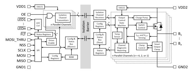
Figure 2. SPI Sourcing Device System Diagram
