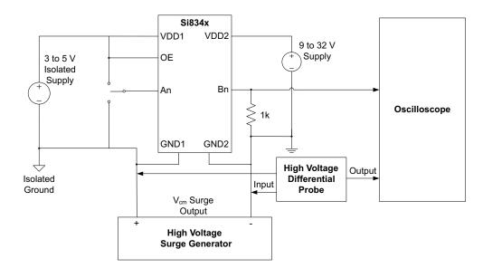
Figure 27. Common Mode Transient Immunity (CMTI) Test Circuit
