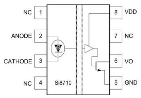
Figure 12. Pin Configuration
