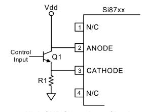
Figure 9. High CMR Si87xx Input Circuit
