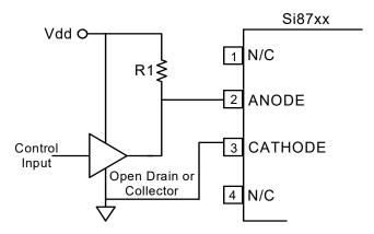
Figure 8. Si87xx Input Circuit
