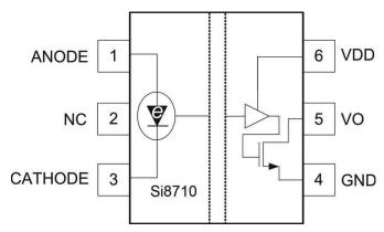
Figure 14. Pin Configuration
