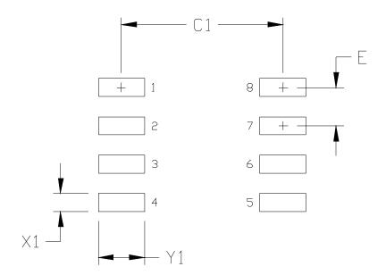
Figure 17. 8-Pin Narrow Body SOIC Land Pattern
