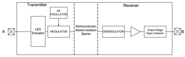
Figure 6. Simplified Channel Diagram
