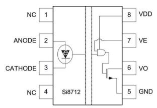
Figure 13. Pin Configuration
