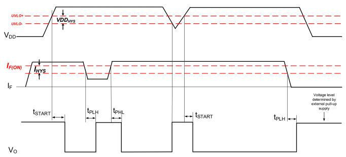
Figure 7. Si87xx Operating Behavior  $(I_F \ge I_{F(MIN)})$  when  $V_F \ge V_{F(MIN)}$
