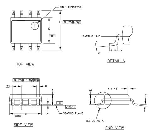
Figure 16. 8-Pin Narrow Body SOIC Package
