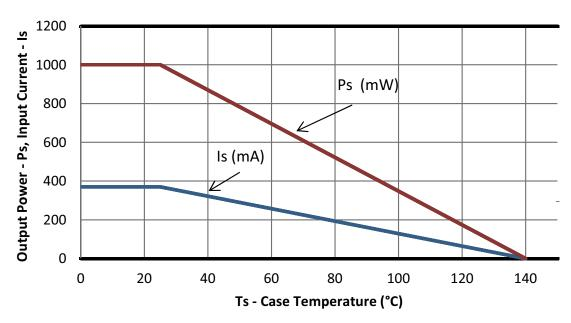
Figure 3. (SOIC-8) Thermal Derating Curve, Dependence of Safety Limiting Values with Case Temperature per VDE0884 part 10
