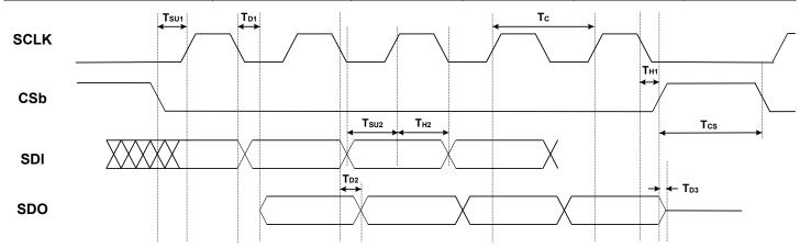
Figure 5.2. 4-Wire SPI Serial Interface Timing
