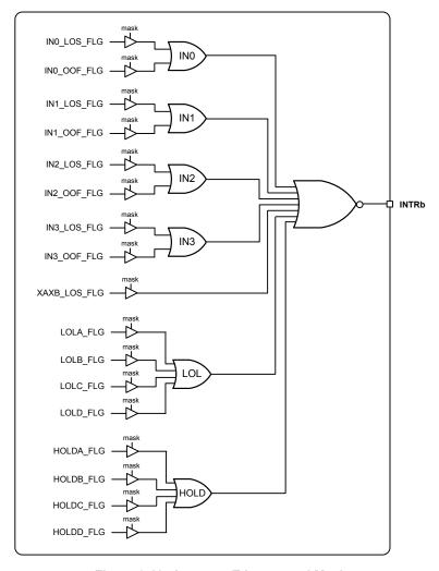
Figure 3.13. Interrupt Triggers and Masks
