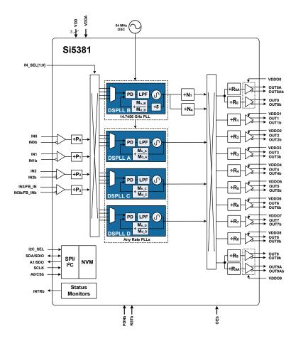
Figure 7.1. Si5381 Block Diagram
