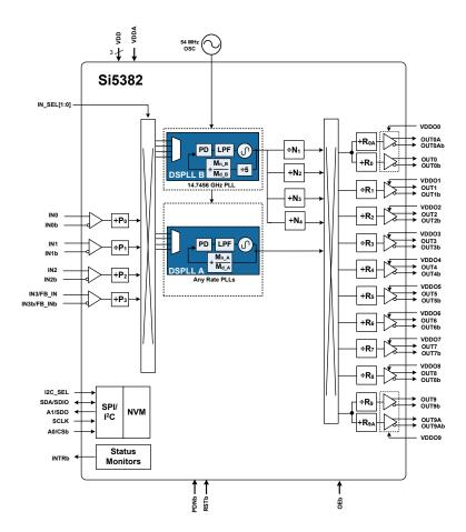
Figure 7.2. Si5382 Block Diagram
