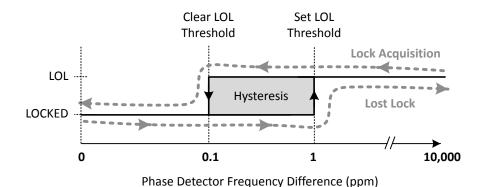
Figure 3.12. LOL Set and Clear Thresholds
