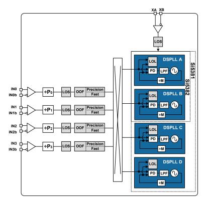
Figure 3.7. Si5381/82 Fault Monitors
