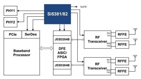
Figure 6.1. Application Block Diagram of µBTS
