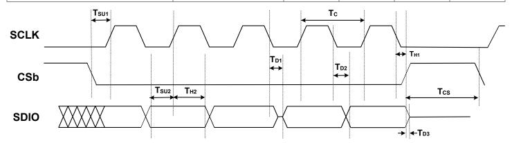
Figure 5.3. 3-Wire SPI Serial Interface Timing
