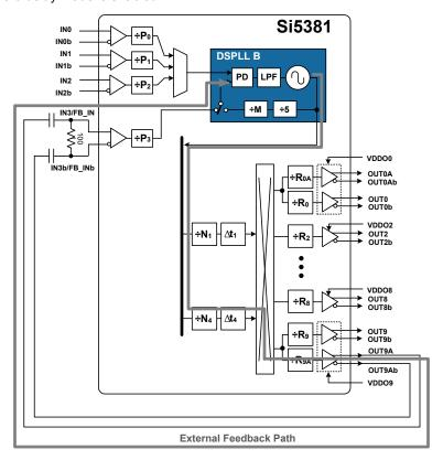
Figure 3.16. Si5381 Zero Delay Mode Setup
