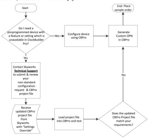
Figure 3.17. Process for Requesting Non-Standard CBPro Features
