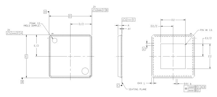
Figure 10.1. Si5381/82 9x9 mm 64-QFN Package Diagram
