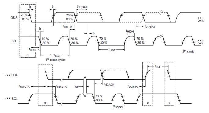
Figure 5.1. I<sup>2</sup>C Serial Port Timing Standard and Fast Modes
