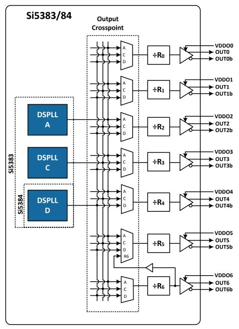
Figure 3.17. DSPLL to Output Driver Crosspoint
