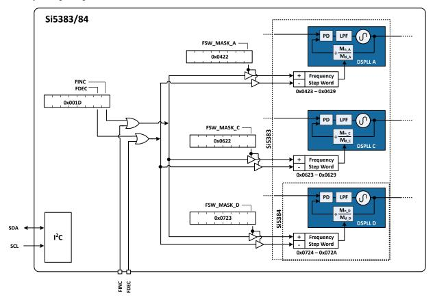
Figure 3.3. Controlling the DCO Mode By Pin Control
