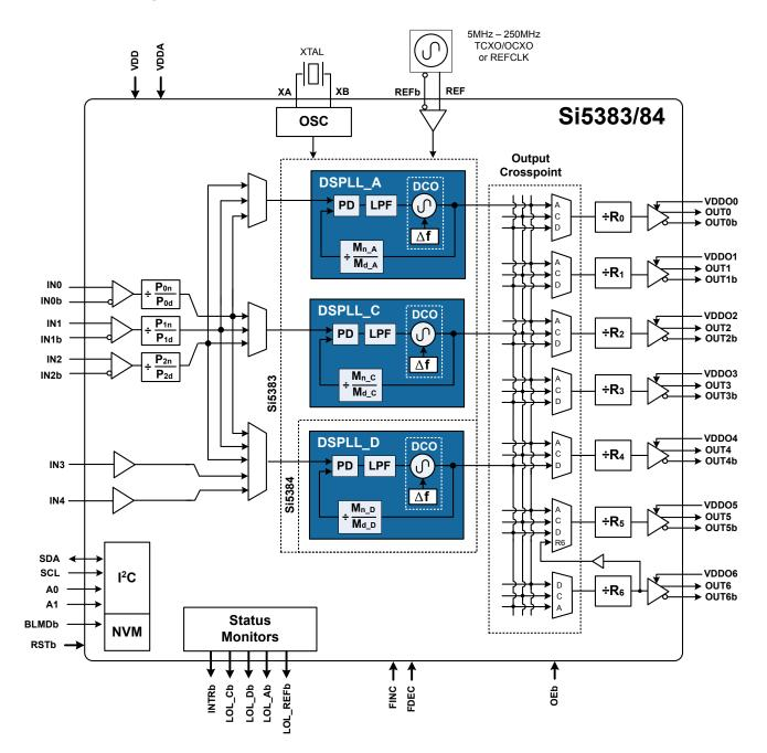
Figure 7.1. Si5383/84 Detailed Block Diagram
