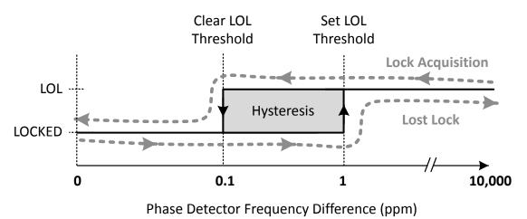
Figure 3.15. LOL Set and Clear Thresholds
