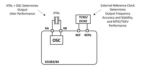
Figure 3.4. External Reference Connections
