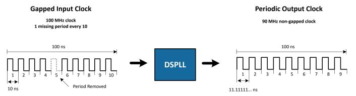
Figure 3.9. Generating an Averaged Clock Output Frequency from a Gapped Clock Input
