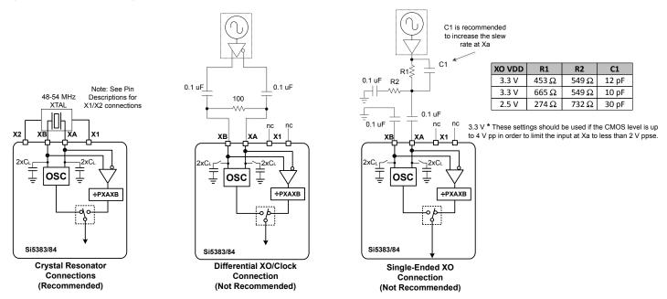
Note: XA and XB must not exceed the maximum input voltage listed in Data Sheet Table Input Clock Specifications
