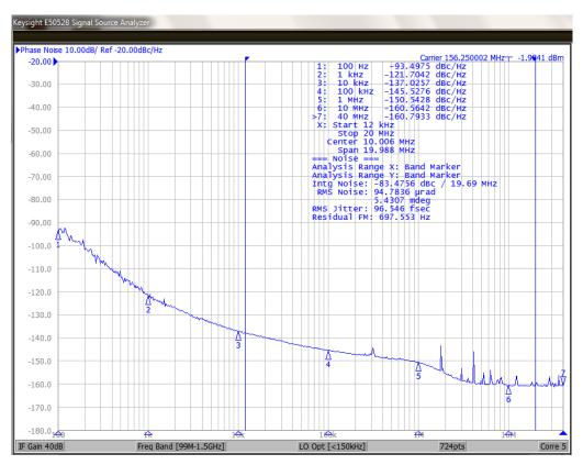
Figure 8.1. F<sub>IN</sub> = 19.44 MHz; F<sub>OUT</sub> = 156.25 MHz, 3.3 V LVPECL with Rakon 12.8 MHz Reference, 48 MHz Crystal
