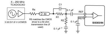
When 3.3 V LVCMOS driver is present, use R2 = 845 ohm and R1 = 267 ohm if needed to keep the signal at INx < 3.6 Vpp\_se. Including C1 = 6 pf may improve the output jitter due to faster input slew rate at INx. If attenuation is not needed for Inx<3.6 Vppse, make R1 = 0 ohm and omit C1, R2 and the capacitor below R2. \* This cap should have less than ~20 ohms of capacitive reactance at the clock input frequency.
