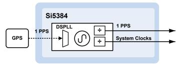
Figure 6.4. Si5384 as a 1 Hz/1 PPS Clock Multiplier
