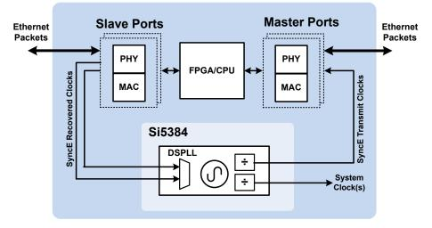
Figure 6.2. Si5384 as a SyncE Jitter/Wander Attenuator
