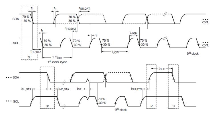
Figure 5.3. I<sup>2</sup>C Serial Port Timing Standard and Fast Modes
