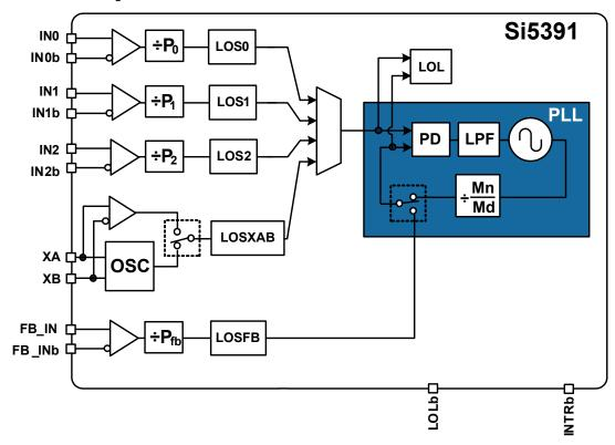
Figure 4.4. LOS and LOL Fault Monitors
