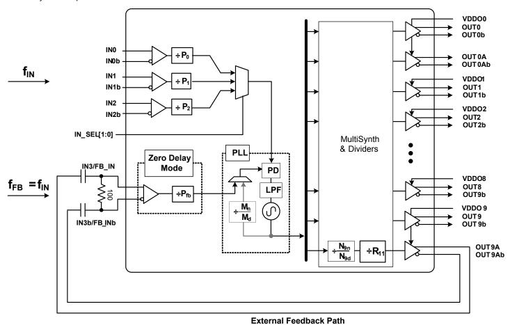
Figure 4.7. Si5391 Zero Delay Mode Setup
