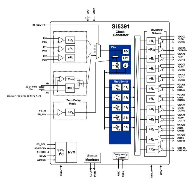
Figure 7.1. Si5391 Block Diagram
