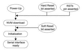
Figure 4.1. Si5391 Power-Up and Initialization
