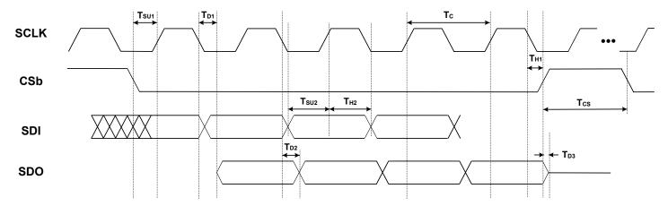
Figure 6.2. 4-Wire SPI Serial Interface Timing
