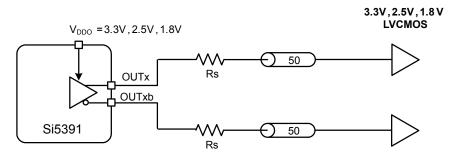
Figure 4.6. LVCMOS Output Terminations
