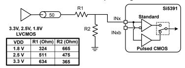
Figure 4.3. Termination of Differential and LVCMOS Input Signals
