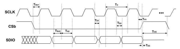
Figure 6.3. 3-Wire SPI Serial Interface Timing
