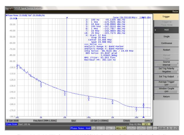
Figure 8.1. 156.25MHz Ouput (3.3V LVPECL) in Precision Calibration Mode (Grade P)
