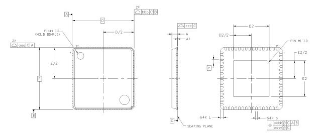
Figure 10.1. 64-Pin Quad Flat No-Lead (QFN)
