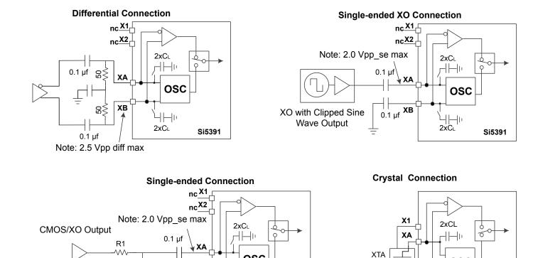
Figure 4.2. XAXB External Crystal and Clock Connections
