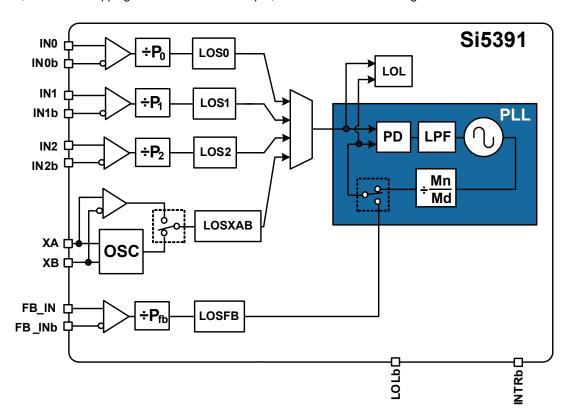
Figure 7.5. Fault Monitors
