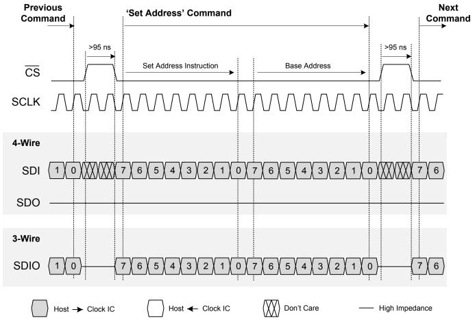
Figure 11.9. SPI "Set Address" Command Timing
