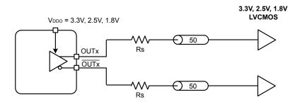
Figure 8.4. LVCMOS Output Terminations
