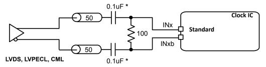
\* These caps should have < ~5 ohms capacitive reactance at the clock input frequency.
