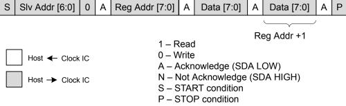
Figure 11.4. I<sup>2</sup>C Write Operation
