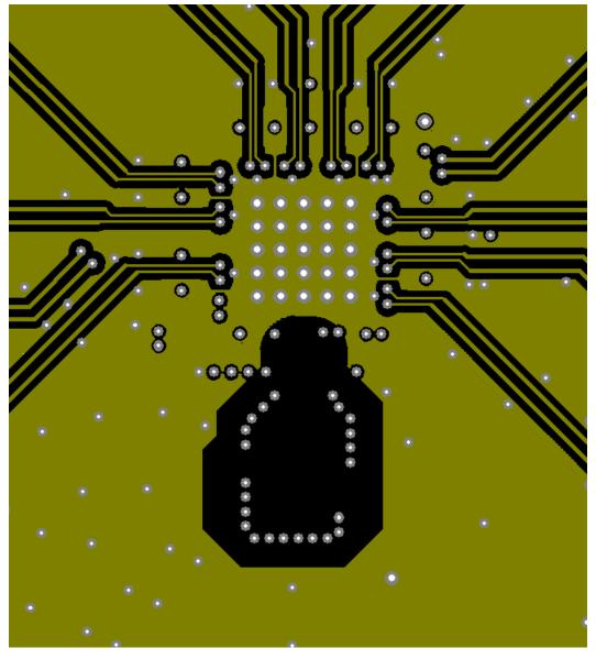
Figure 12.7. Output Clock Layer (Layer 7)
