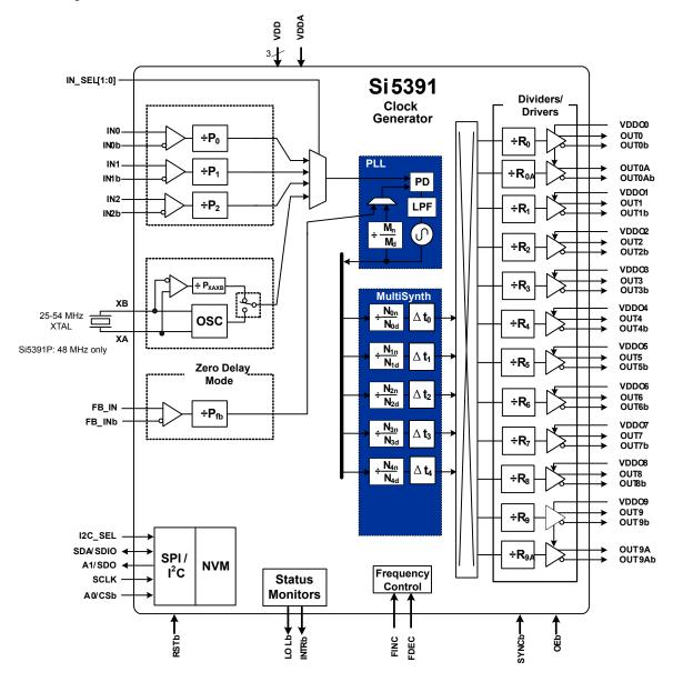
Figure 3.1. Si5391 Block Diagram
