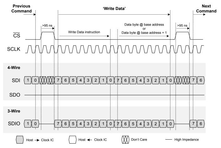
Figure 11.10. SPI "Write Data" and "Write Data+ Address Increment" Instruction Timing
