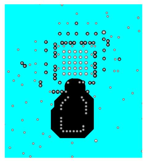
Figure 12.3. Crystal Ground Plane (Layer 3)
