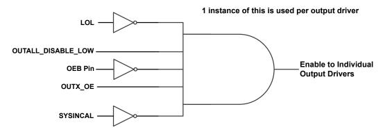
OUTX\_OE are the individual Output Driver enables as shown in the table below
