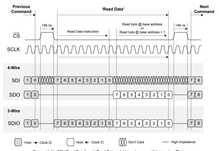
Figure 11.11. SPI "Read Data" and "Read Data + Address Increment" Instruction Timing
