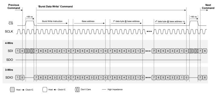
Figure 11.12. SPI "Burst Data Write" Instruction Timing
