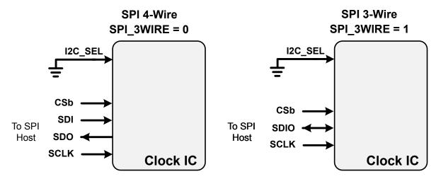
Figure 11.6. SPI Interface Connections
