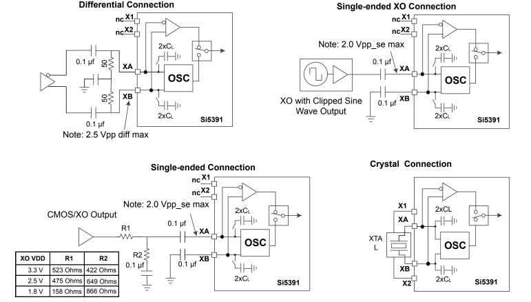
Figure 7.2. Crystal Resonator and External Reference Clock Connection Options
