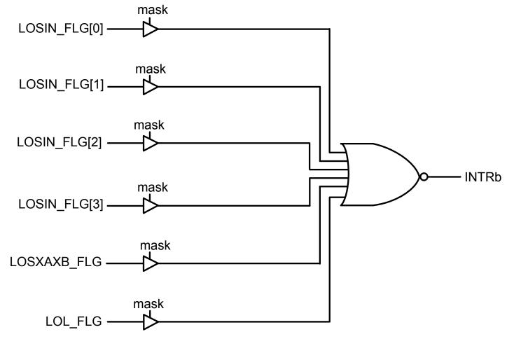
Figure 7.6. Interrupt Triggers and Masks
