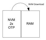
Figure 4.2. Si5391/Si5391P Memory Configuration
