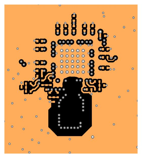
Figure 12.8. Bottom Layer Ground Flooded (Layer 8)
