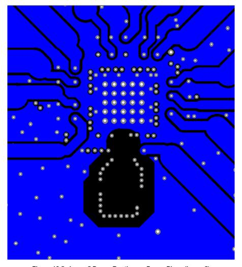
Figure 12.5. Layer 5 Power Routing on Power Plane (Layer 5)
