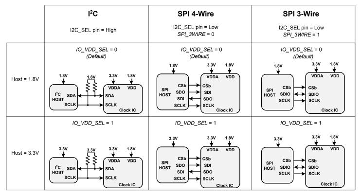
Figure 11.1. I<sup>2</sup>C/SPI Device Connectivity Configurations
