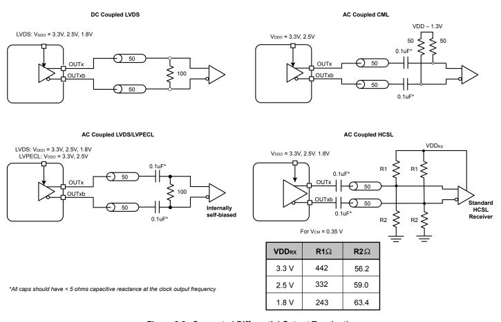
Figure 8.2. Supported Differential Output Terminations
