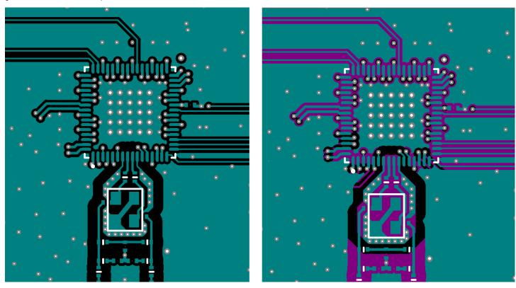
Figure 12.1. 64-pin Si5391/Si5391P Crystal Layout Recommendations Top Layer (Layer 1)
