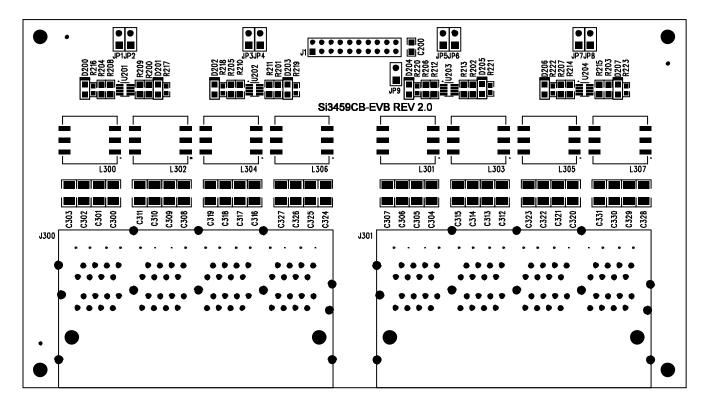
Figure 28. Connector Board Top Silkscreen
