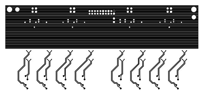
Figure 30. Connector Board Ground Layer
