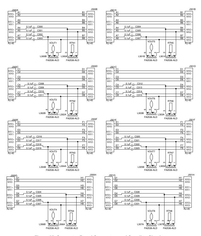
Figure 27. Connector Board Connectors and Coupling Circuits
