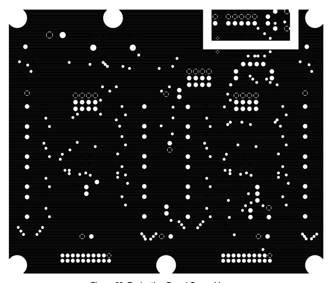
Figure 22. Evaluation Board Ground Layer
