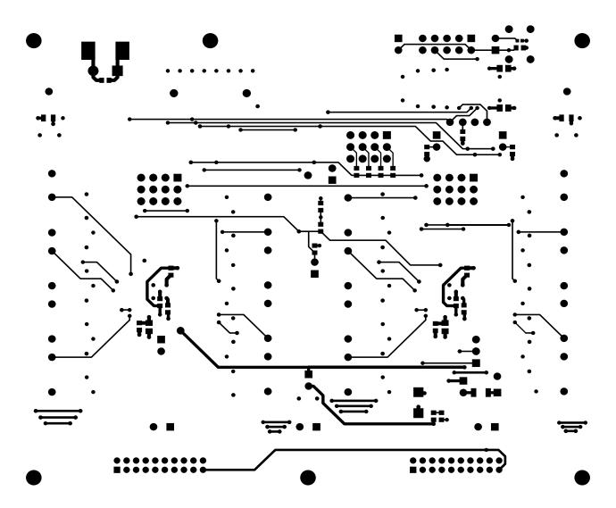
Figure 24. Evaluation Board Bottom Side
