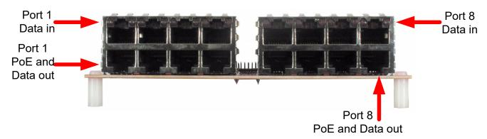
Figure 7. Connector Board Configuration
