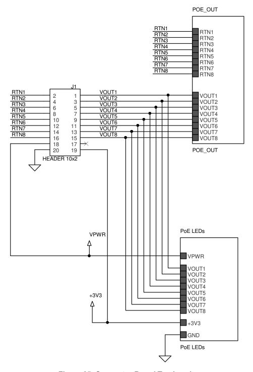
Figure 25. Connector Board Top Level
