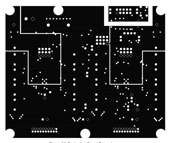
Figure 23. Evaluation Board Power Layer
