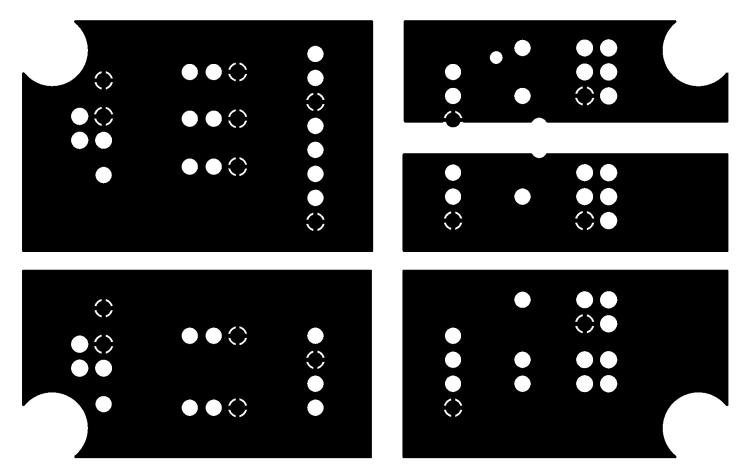
Figure 5.3. Si827x Layer 3: Power Plane
