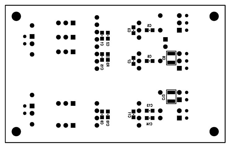
Figure 3.2. Si827x Evaluation Board Secondary Silkscreen
