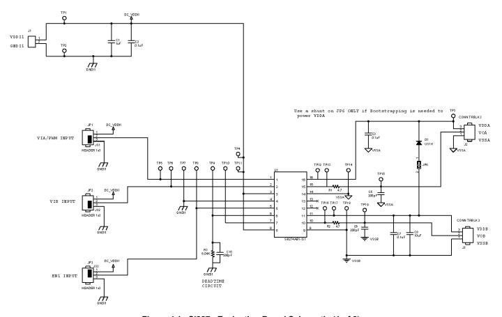
Figure 4.1. Si827x Evaluation Board Schematic (1 of 2)
