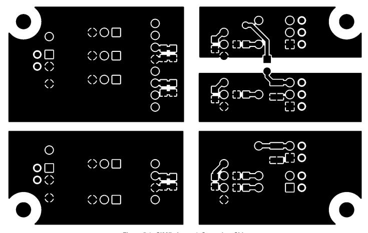
Figure 5.4. Si827x Layer 4: Secondary Side
