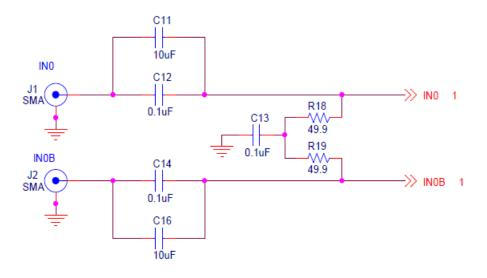
Figure 5.2. Differential Clock Input Terminations
