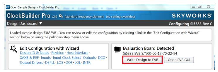
Figure 6.10. Write Design to EVB
