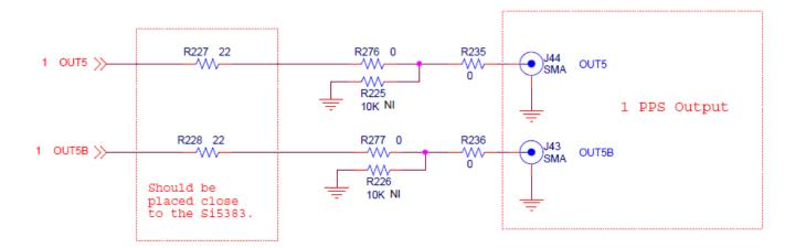
Figure 5.5. OUT5 Termination Circuit
