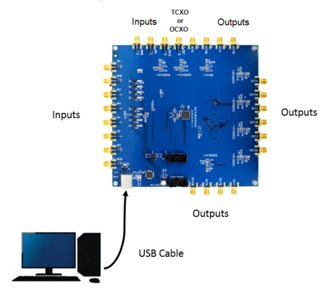
Figure 6.1. EVB Connection Diagram
