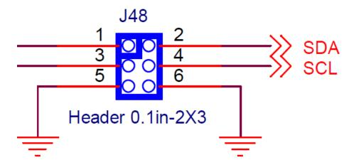
Figure 8.1. Serial Communications Header J48
