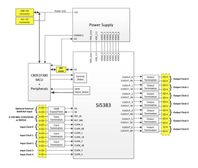
Figure 1.1. Si5383-EVB Functional Block Diagram
