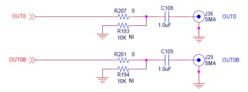
Figure 5.4. Output Clock Termination Circuit
