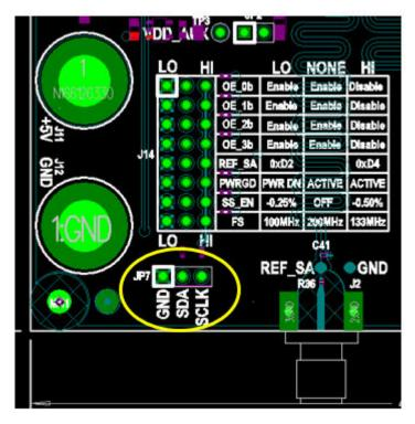
Figure 7.1. I2C Access Header Location
