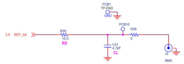
Figure 4.2. Reference Output Clock Termination
