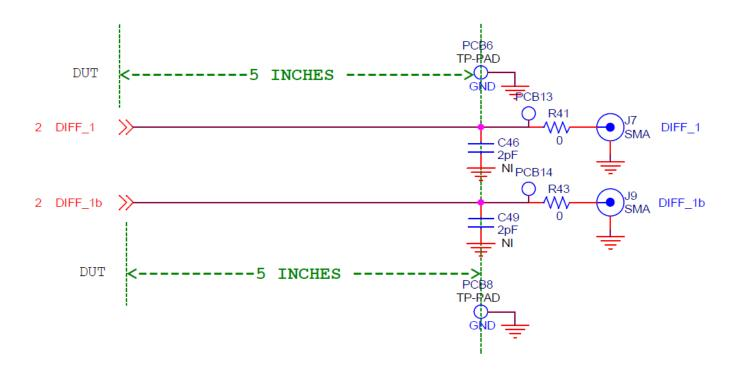
Figure 4.1. Differential Output Clock Termination
