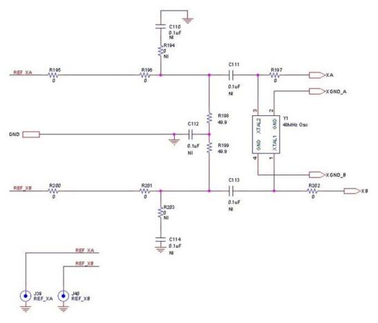
Figure 6.1. External Reference Input Circuit
