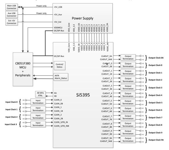
Figure 1.1. Si5395 EB Functional Block Diagram
