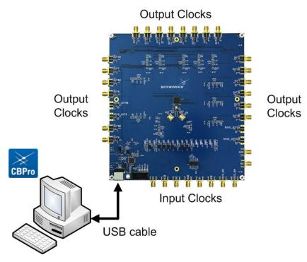
Figure 10.1. EVB Connection Diagram
