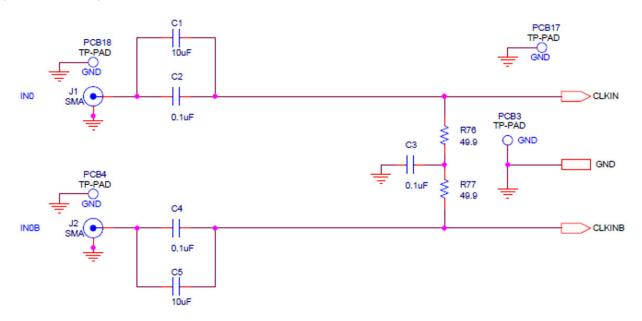
Figure 7.1. Input Clock Termination Circuit
