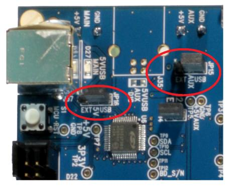
Figure 10.2. JP15–JP16 Standard Jumper Shunt Installation
