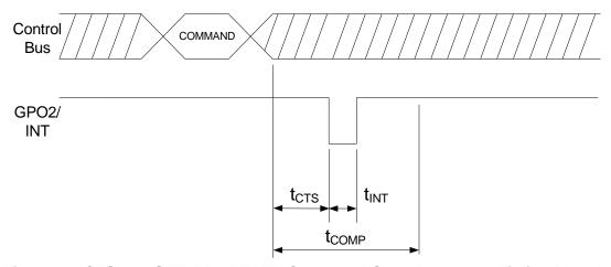
Figure 30. CTS and SET\_PROPERTY Command Complete  $t_{\text{COMP}}$  Timing Model
