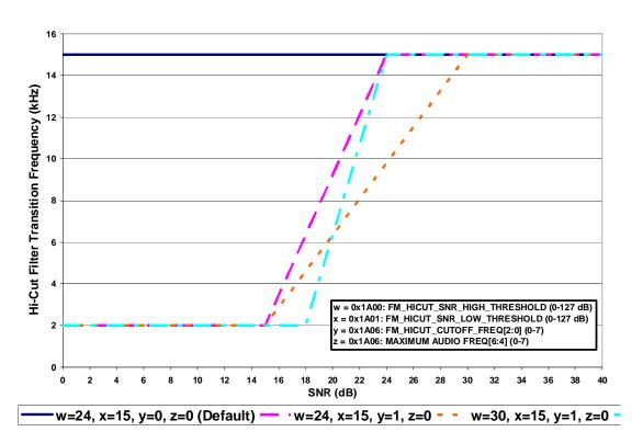
Figure 8. HiCut Controlled by SNR Metric
