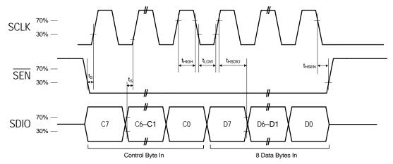
Figure 21. SPI Control Interface Write Timing Parameters
