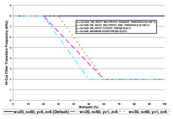
Figure 11. HiCut Controlled by Multipath Metric with Maximum Audio Frequency 8 kHz
