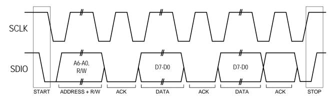
Figure 18. 2-wire Control Interface Read and Write Timing Diagram
