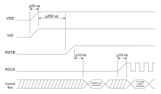
Figure 23. Device Power Up Timing
