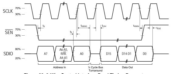
Figure 20. 3-Wire Control Interface Read Timing Parameters
