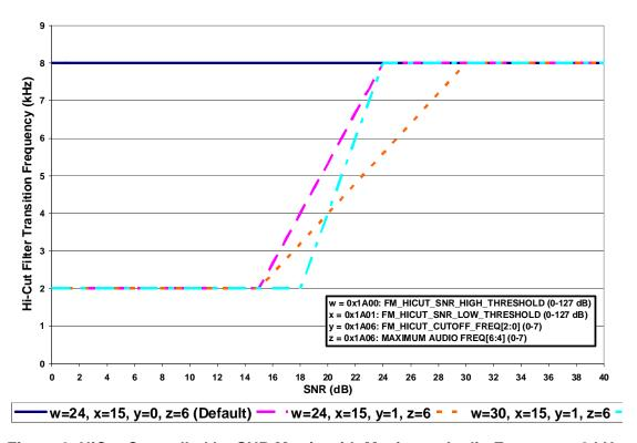
Figure 9. HiCut Controlled by SNR Metric with Maximum Audio Frequency 8 kHz
