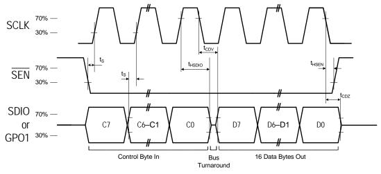
Figure 22. SPI Control Interface Read Timing Parameters
