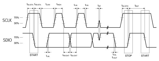
Figure 17. 2-wire Control Interface Read and Write Timing Parameters
