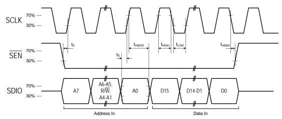
Figure 19. 3-Wire Control Interface Write Timing Parameters
