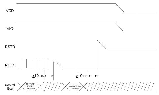
Figure 24. Device Power Down Timing
