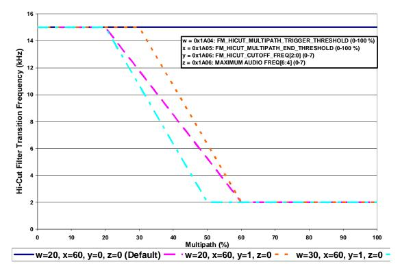
Figure 10. HiCut Controlled by Multipath Metric
