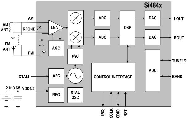
Figure 4. Si4840/44-A10 Functional Block Diagram
