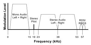
Figure 5. MPX Signal Spectrum
