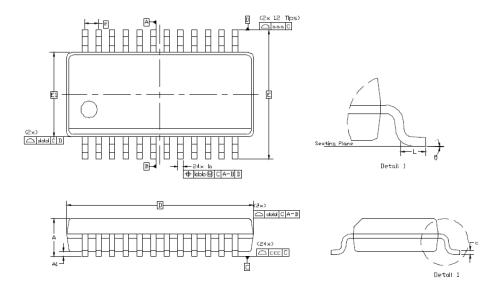
Figure 6. 24-Pin SSOP
