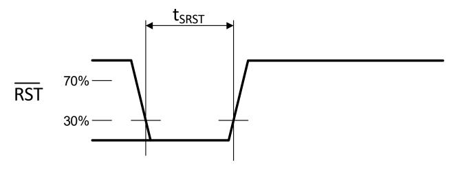
Figure 1. Reset Timing
