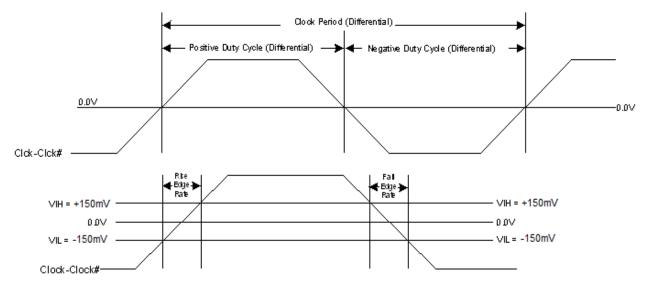
Figure 4. Differential Output Signals (for AC Parameters Measurement)
