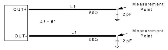
Figure 3. 0.7 V Differential Load Configuration
