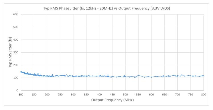
Phase jitter measured with Agilent E5052 using a differential-to-single ended converter (balun or buffer). Measurements collected for >700 commonly used frequencies. Phase noise plots for specific frequencies are available using our onlineOscillator Phase Noise Lookup Tool.
