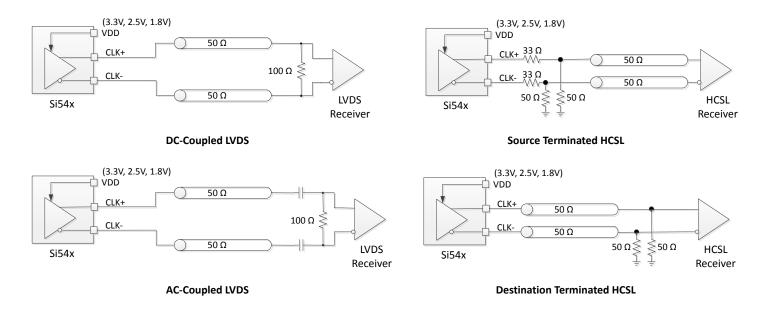
Figure 4.2. LVDS and HCSL Output Terminations
