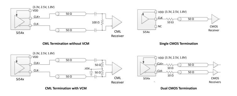
Figure 4.3. CML and CMOS Output Terminations
