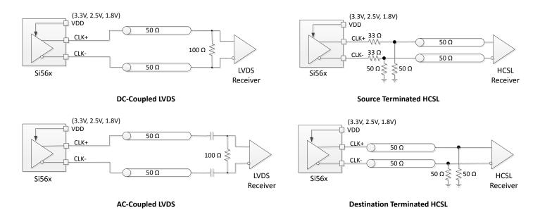
Figure 4.2. LVDS and HCSL Output Terminations
