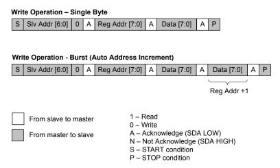
Figure 5.3. I2C Write Operation
