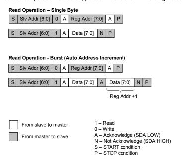
Figure 5.4. I2C Read Operation
