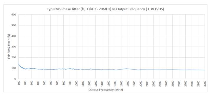
Figure 2.2. Phase Jitter vs. Output Frequency
