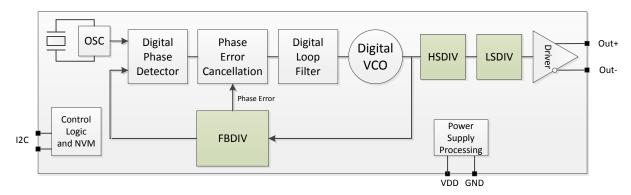
Figure 5.2. Si564 Frequency Definition Block Diagram
