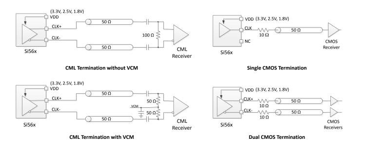
Figure 4.3. CML and CMOS Output Terminations
