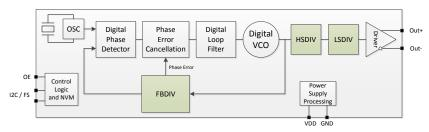
Figure 5.1. Si564 Block Diagram
