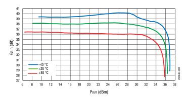
Figure 7. Gain vs Pout Across Frequency
