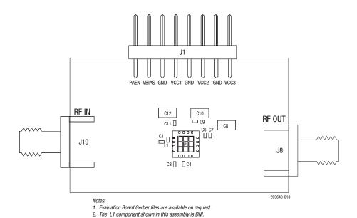
**Figure 18. Evaluation Board Assembly Drawing**
