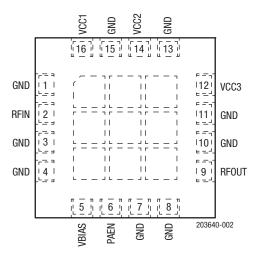
Figure 2. SKY66394-11 Pinout (Top View)
