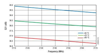
Figure 13. Small Signal Gain vs Frequency Across Temperature  $(P_{IN} = -30 \text{ dBm})$
