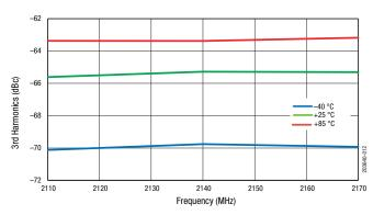
Figure 12. 3<sup>rd</sup> Harmonic vs Frequency Across Temperature @ Pout = +28 dBm(GW)
