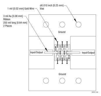
Figure 4. Suggested Die Mount and Ribbon Attachment  $(\geq 6 \text{ dB})$
