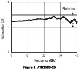
Typical Insertion Loss vs Frequency
