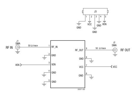
Figure 3. SKY65720-11 Evaluation Board Schematic
