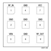
Figure 2. SKY65720-11 Pinout (Top View)
