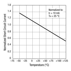
Figure 5. Normalized Short Circuit Current vs Temperature
