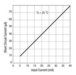
Figure 3. Short Circuit Current vs Input Current
