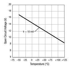
Figure 6: Open Circuit Voltage vs Temperature
