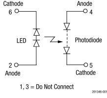
Figure 1. OLS910 Block Diagram
