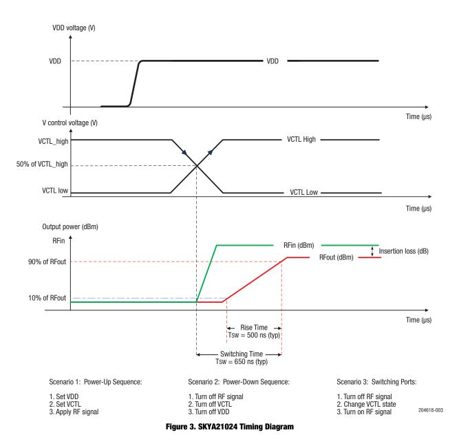
**Typical Performance Characteristics** (VDD = 2.8 V, VCTL = 1.8 V, TOP = +25 °C, PIN = 0 dBm, Characteristic Impedance [Zo] = 50  $\Omega$ , Unless Otherwise Noted)
