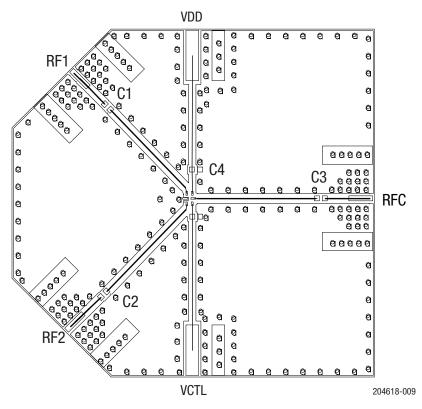
Figure 9. SKYA21024 Evaluation Board Assembly Diagram
