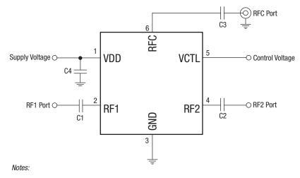
C1, C2, and C3 = 10 nF for low frequency applications (less than 100 MHz) C4 = 10 nF
